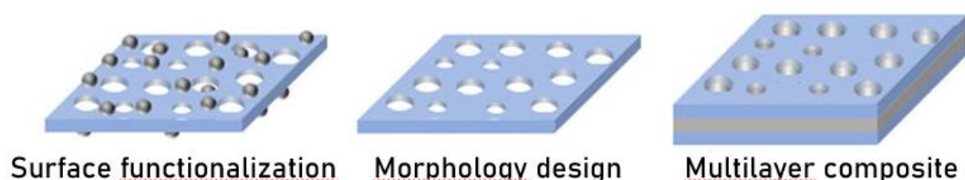
Figure 2.7 Three examples representing modification methods to design functional separators
