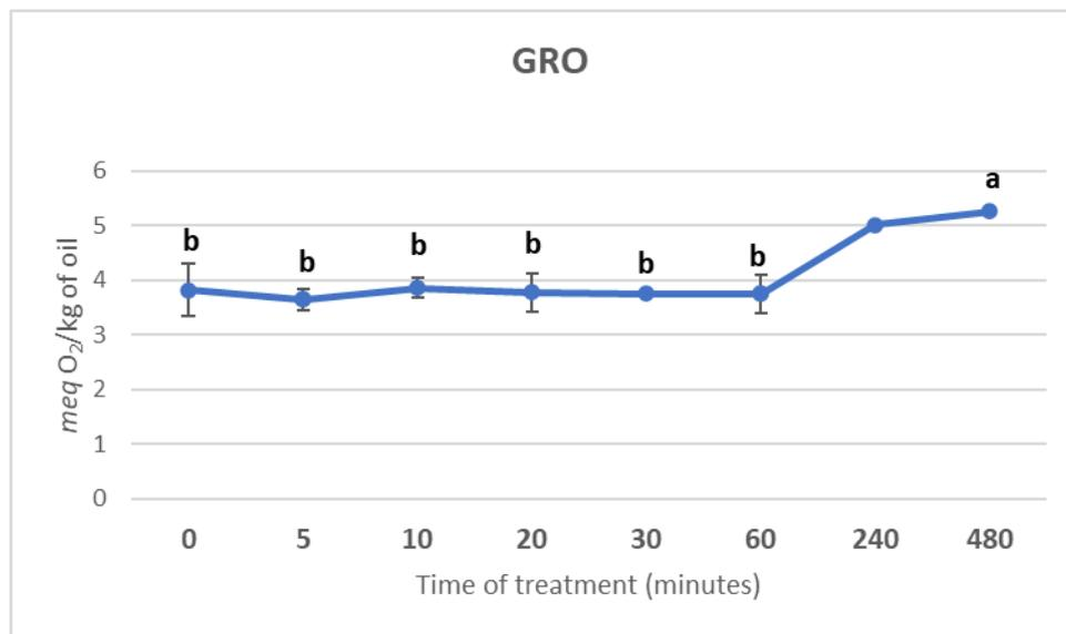
Figure 4.30. Graphical representation of the trend in peroxide value (PV) over time for the grapeseed oil (GRO) sample, expressed as meq O<sub>2</sub>/kg of oil. Data points with different letters at various treatment times are significantly different ( $p \leq 0.05$ ).
