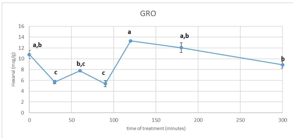
Figure 4.13. Graphical representation of the trend in hexanal content over time for the grapessed oil (GRO) sample, expressed as area. Data points labelled with different letters at various thermal treatment times are significantly different ( $p \leq 0.05$ ).
