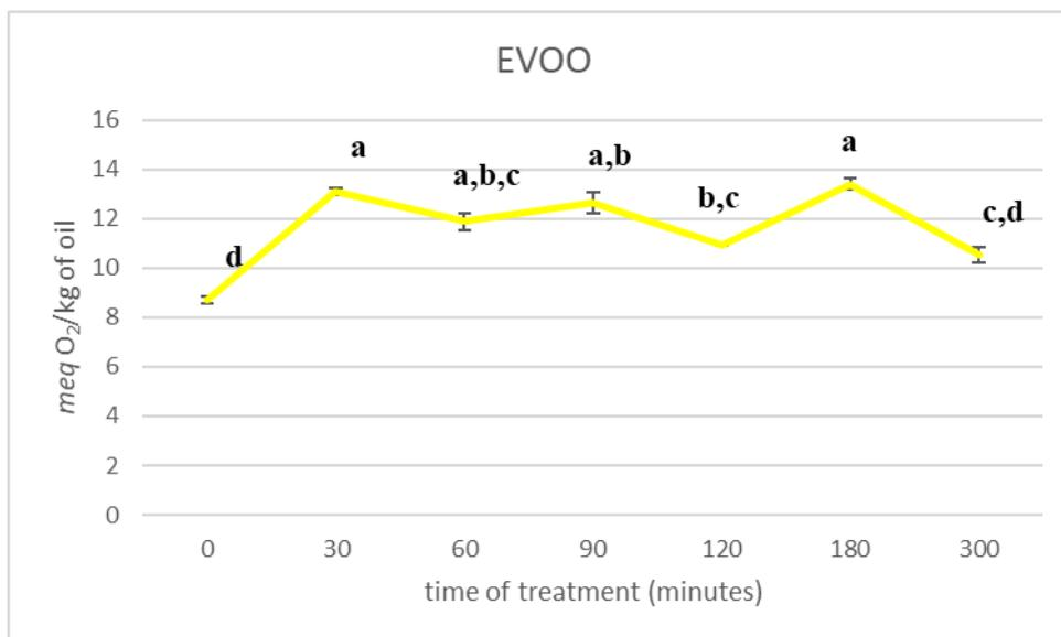
Figure 4.6. Graphical representation of the trend in peroxide value over time for the extra-virgin olive oil (EVOO) sample, expressed as meq O<sub>2</sub>/kg of oil. Data points labelled with different letters for the various thermal treatment times are significantly different ( $p \leq 0.05$ )
