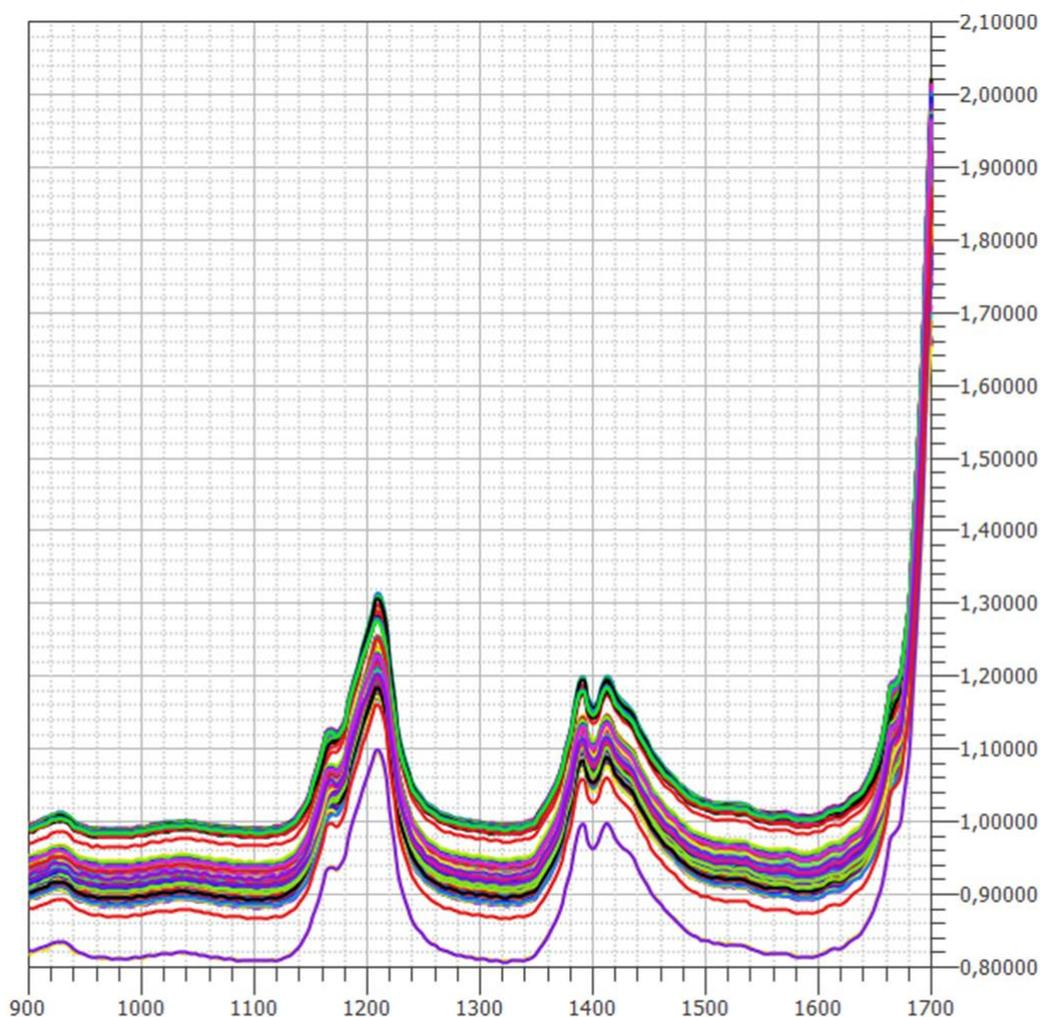
Figure 4.75. Raw signal of all the samples analysed, it is possible to see how the regions between 1140÷1260, 1360÷1480 and over 1700 nm tend to give same behaviour all over the different kinds of samples considered.
