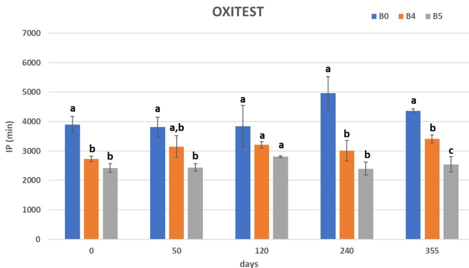
Figure 4.73. Comparison of IP values among B0, B4, and B5 obtained by performing the analysis at  $T = 90^{\circ}\text{C}$  and a pressure of 6 bar. Bars with different letters within each category are significantly different ( $p \leq 0.05$ ).
