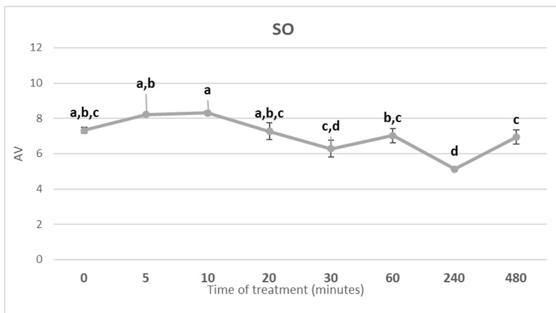
Figure 4.41. Graphical representation of the trend in anisidine value over time for the sunflower oil (SO) sample. Data points labelled with different letters at various thermal treatment times are significantly different ( $p \leq 0.05$ ).
