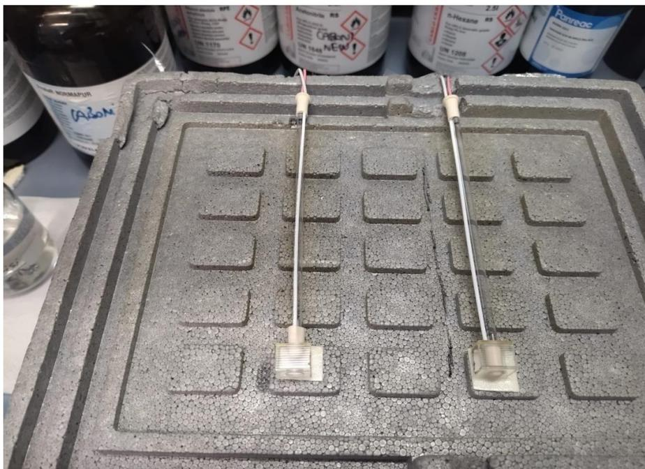
Figure 3.3. Internal view of the lid, the lamps were mounted inside the chamber with as little external contamination as possible.
