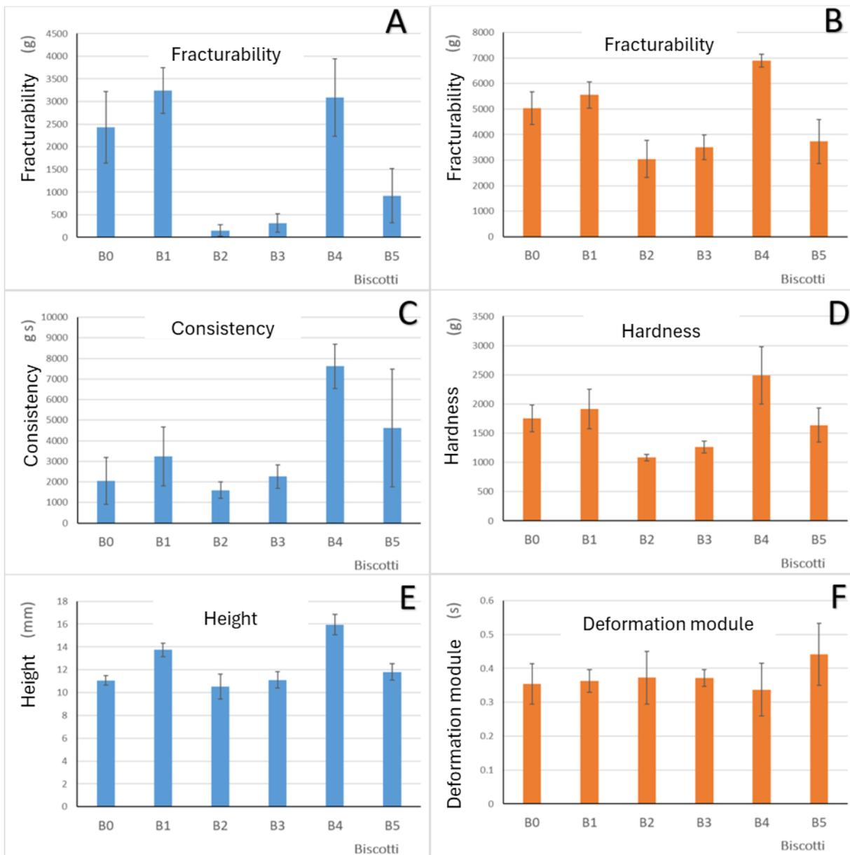
Figure 4.59. Results from the penetrability test (A,C,E) and the break test (B,D,F)
