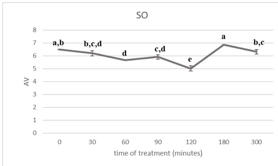
Figure 4.20. Graphical representation of the trend in Anisidine value content over time for the sunflower oil (SO) sample, expressed as AV. Data points labelled with different letters at various thermal treatment times are significantly different ( $p \leq 0.05$ ).
