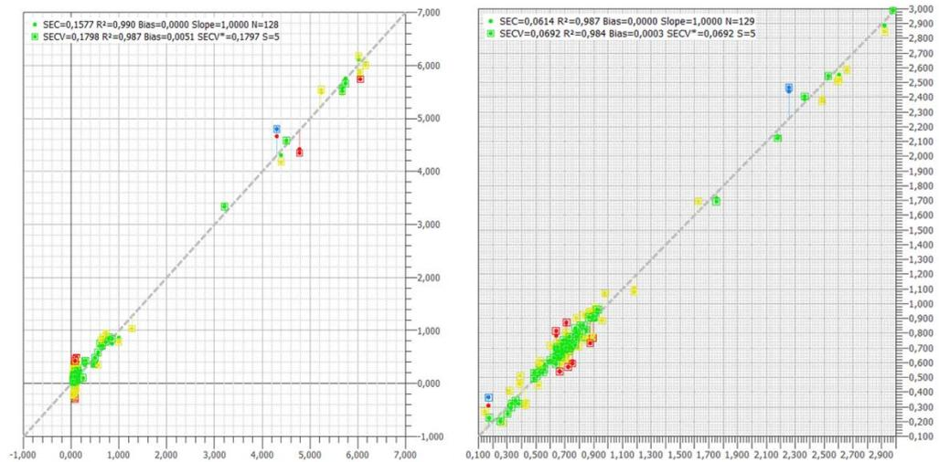
Figure 4.78 and 5.79. Regression models for the linolenic and beenic acids, it is clearly observable how the models may result in high, theoretical, descriptive accuracy, however the missing of intermediate points along the regression model leads to high standard errors, which impair the accuracy of the prediction.
