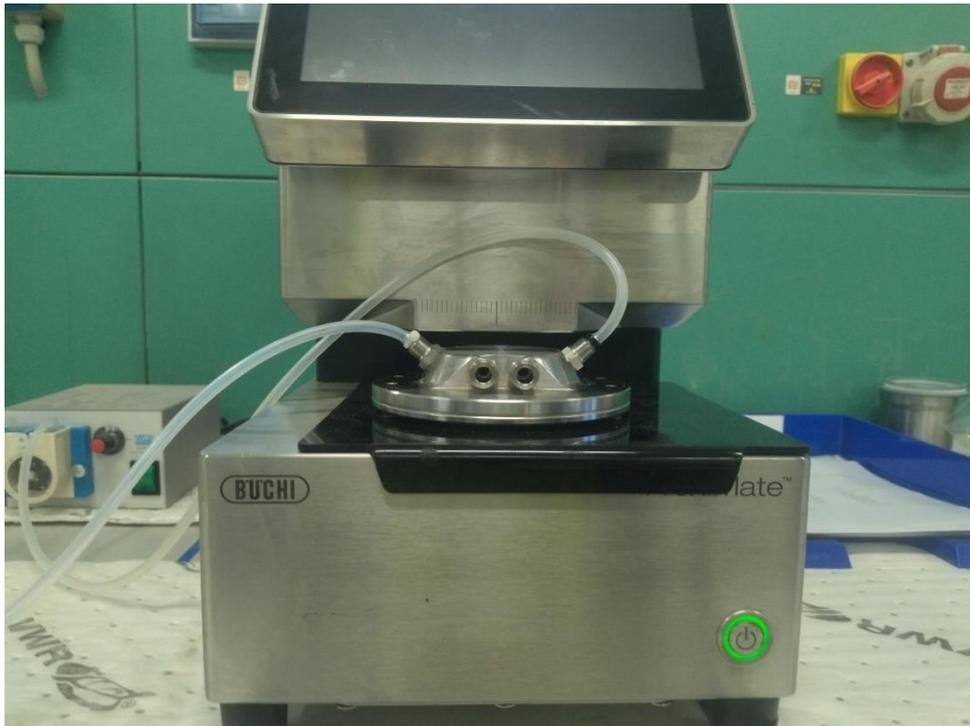
*Figure 3.4. Flux camber prototype implemented in the NIR analysis of the oils, the samples were charged by a peristaltic pump with the hose on the left side of the image and discharged through the right one. The prototype also worked as the transmittance medium.*
