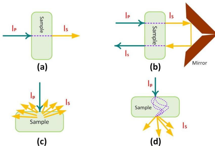
Figure 1.20. (a) Transmittance measurement mode, which is used with gases and semi-solids placed in a cuvette; (b) transflectance measurement mode, which is used with semi-solids without a cuvette; (c) diffuse reflectance measurement mode, which is used with solids where the measurement is taken from the NIR incidence; (d) transmittance through a scattering medium (Zhang et al., 2022).
