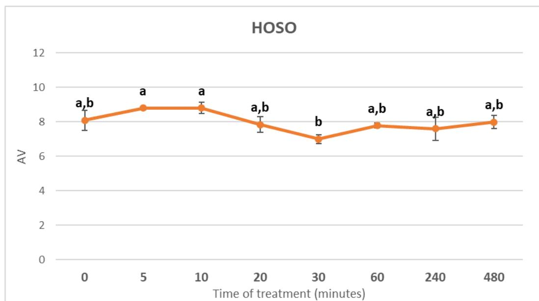
Figure 4.40. Graphical representation of the trend in anisidine value over time for the high-oleic sunflower oil (HOSO) sample. Data points labelled with different letters at various thermal treatment times are significantly different ( $p \leq 0.05$ ).
