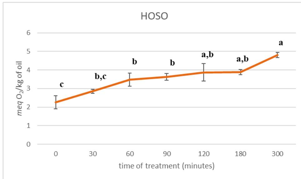
Figure 4.9. Graphical representation of the trend in peroxide value over time for the high-oleic sunflower oil (HOSO) sample, expressed as meq O<sub>2</sub>/kg of oil. Data points labelled with different letters for the various thermal treatment times are significantly different ( $p \leq 0.05$ )
