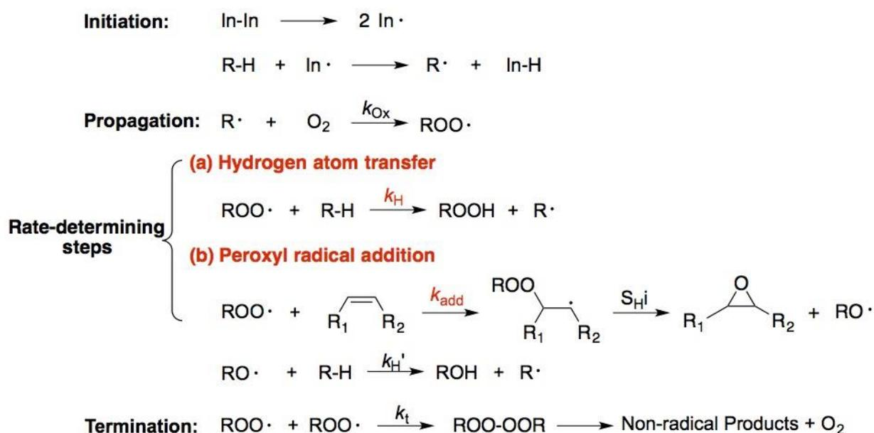
Figure 1.14: Initiation, propagation, and termination of lipid autoxidation.
