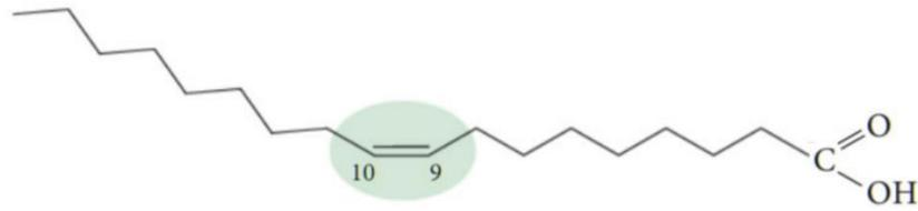
Figure 1.15: Chemical structure of oleic acid.
