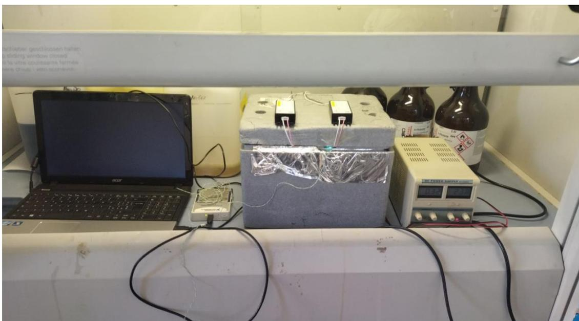
*Figure 3.1. Photo-oxidation system. From left to right, the setup includes: a computer equipped with software for temperature monitoring via thermocouples, the thermocouple system, the oxidation chamber with UV lamps installed above it, and the current transformer.*
