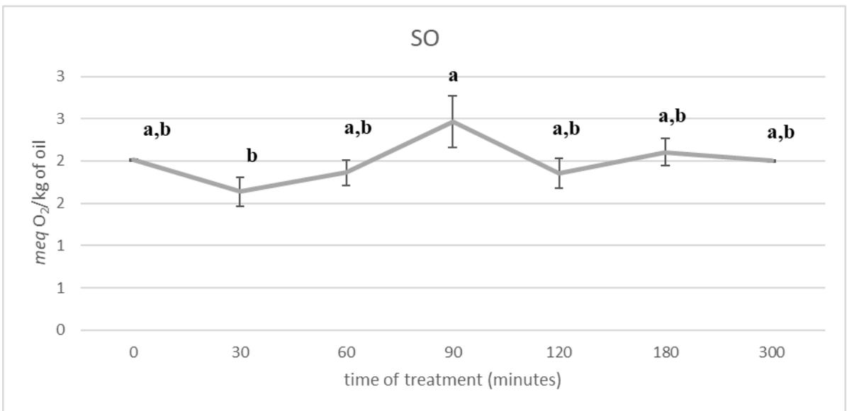
Figure 4.8. Graphical representation of the trend in peroxide value over time for the sunflower oil (SO) sample, expressed as meq O<sub>2</sub>/kg of oil. Data points labelled with different letters for the various thermal treatment times are significantly different ( $p \leq 0.05$ )
