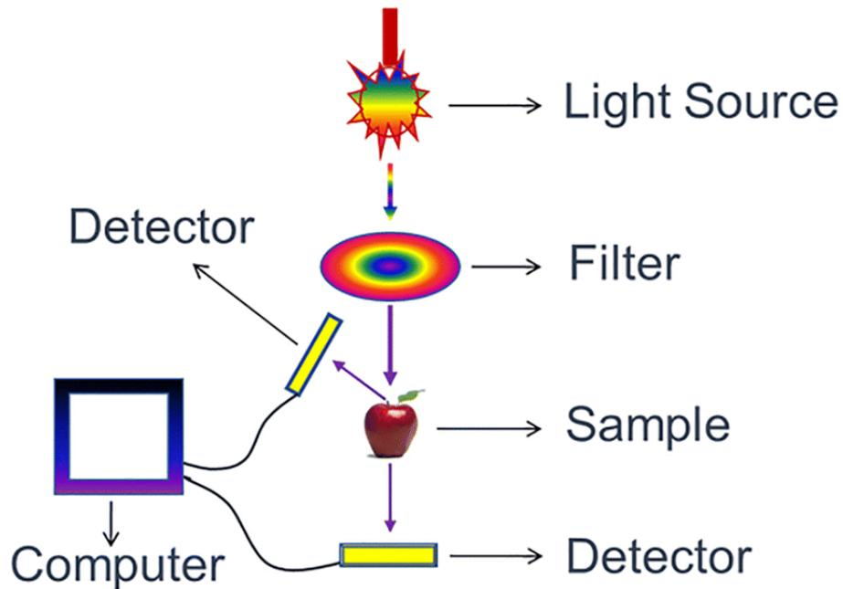
Figure 1.19. Schematic workflow of NIR instrument (Chandrasekaran et al., 2019).
