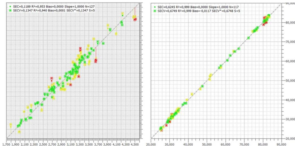
Figure 4.76 and 5.77. Regression models for the stearic and oleic acids, it is possible to observe the almost even distribution of points along the model.
