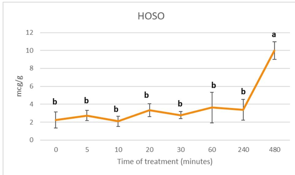
Figure 4.36. Graphical representation of the trend in hexanal content over time for the high-oleic sunflower oil (HOSO) sample, expressed as mcg of hexanal/g. Data points labelled with different letters at various thermal treatment times are significantly different ( $p \leq 0.05$ ).
