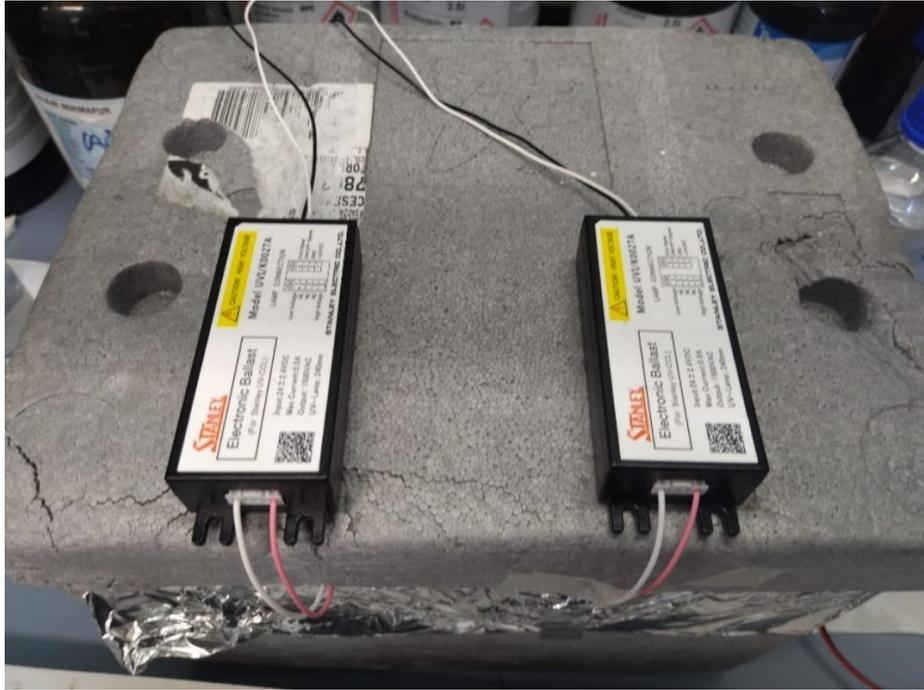
Figure 3.2. External view of the lid, the ballasts were mounted on the external part of the system.
