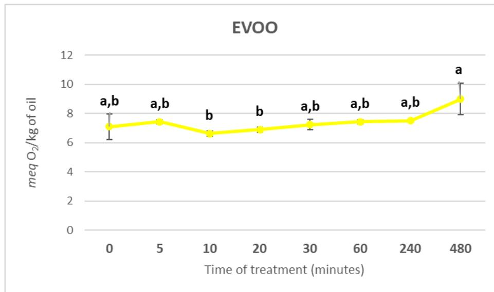
Figure 4.33. Graphical representation of the trend in peroxide value (PV) over time for the extra-virgin olive oil (EVOO) sample, expressed as meq O<sub>2</sub>/kg of oil. Data points with different letters at various treatment times are significantly different ( $p \leq 0.05$ ).
