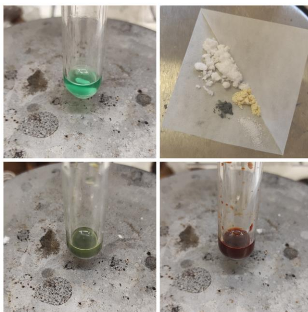
Figure 81. Top Left: [Ni( L5 )Cl 2 ] solution in DMA. Top right: Solid reagents ( 14 , 13p , Zn, NaI). Bottom left: Reaction mixture after addition of all solids. Bottom right: Reaction mixture few seconds after the addition of TMSCl.
