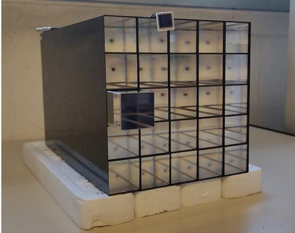
Figure 2.16: The prototype calorimeter, with the 25  $PbWO_4$  crystals and the APD (shown on top) for the readout.
