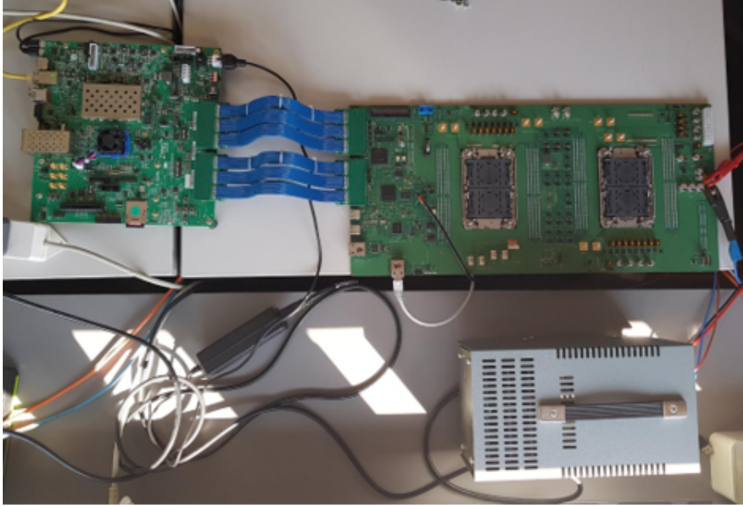
FIGURE 6.4: The EPI LRP (on the right) connected to the FPGA (on the left) executing the HIL framework.
