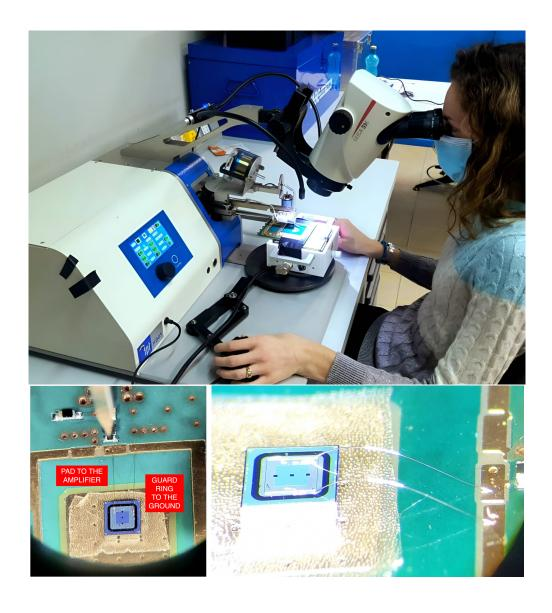
Figure 4.21: Wire bonder (top) and sensor bonded to the front-end board (bottom).
