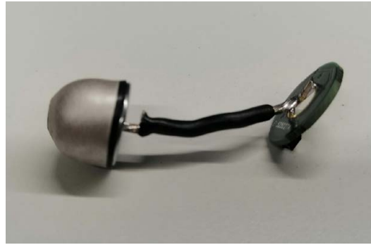
Figure 5.1: Ear-EEG electrode fabricated by Dätwyler Schweiz AG and connected to an active buffering PCB
