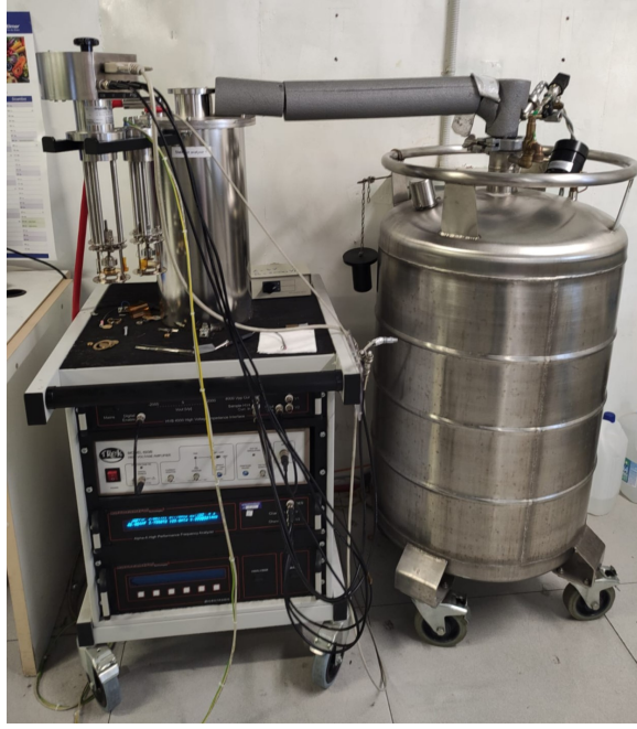
Figure 3.13: Dielectric spectroscopy setup
