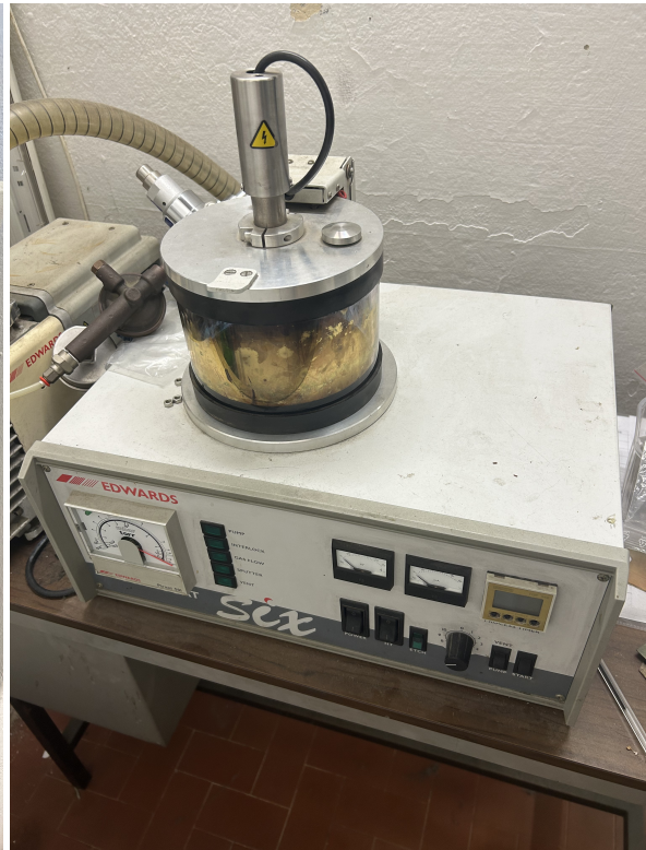
(b) Cold sputtering setup
