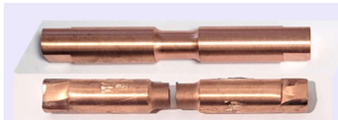
Fig. 2.14 Torsion specimen before and after the test.
