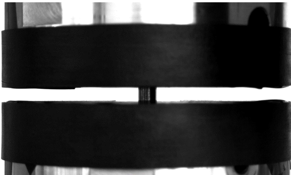
Fig. 2.9 Photo of the ETP Copper compression test performed at the DIN-Department of Industrial Engineering of the University of Bologna.
