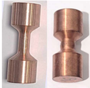
Fig. 2.29 Hybrid-compression specimen before and after the test.
