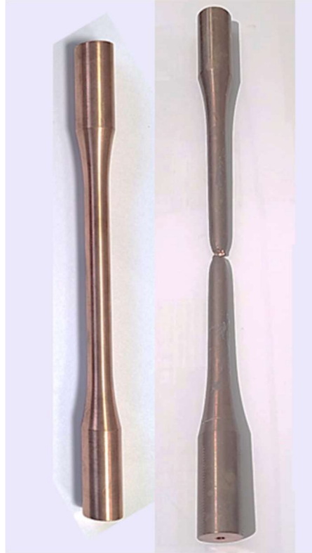
Fig. 2.2 Tensile specimen before and after the test.
