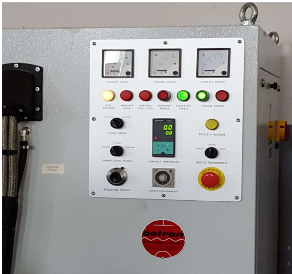
Fig. 1.8 Photo of the Inductive Generator of the Torsion Machine at the DIN-Department of Industrial Engineering of the University of Bologna.
