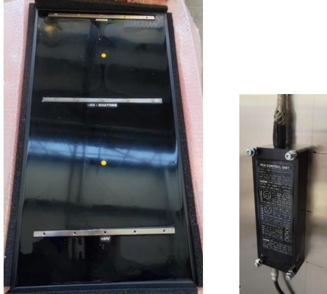
Figure 3.9 – HV SiC switch with its separated control unit
