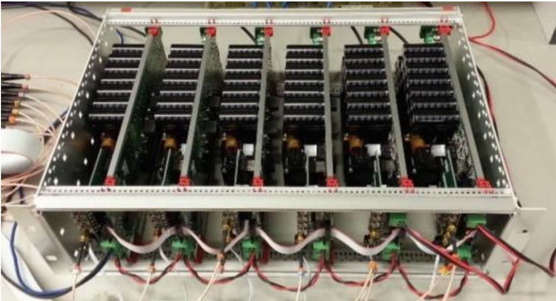
Figure 4.11 - MMC prototype, encompassing six SMs, used for experimental tests.
