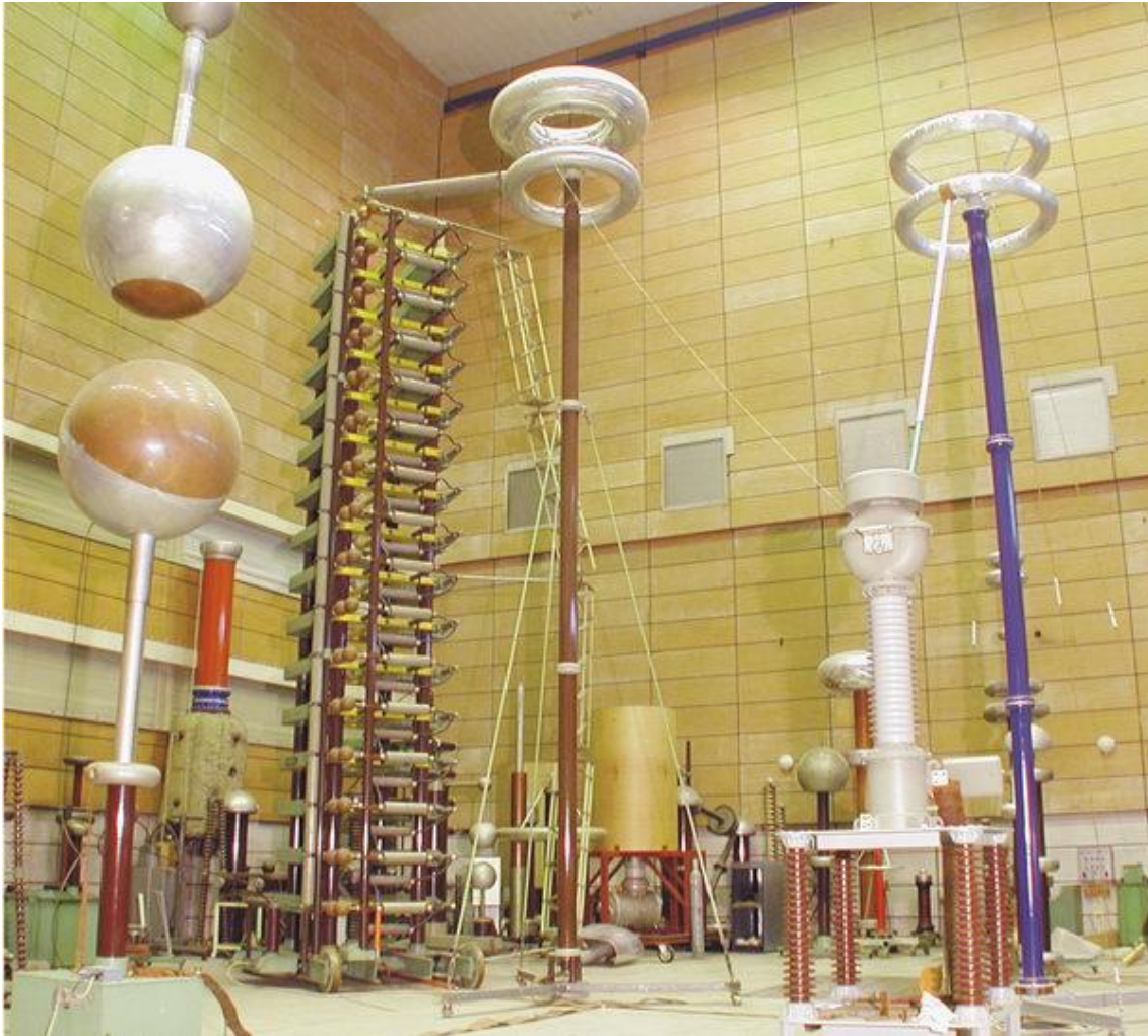
Figure 3.1 – Marx generator built in 1961, currently at the High Voltage laboratory of the Technische Universität Darmstadt [51]
