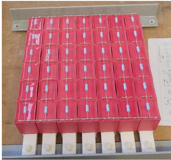
Figure 3.8 – Storage Bank made of 42 capacitors each with a paralleled resistor.
