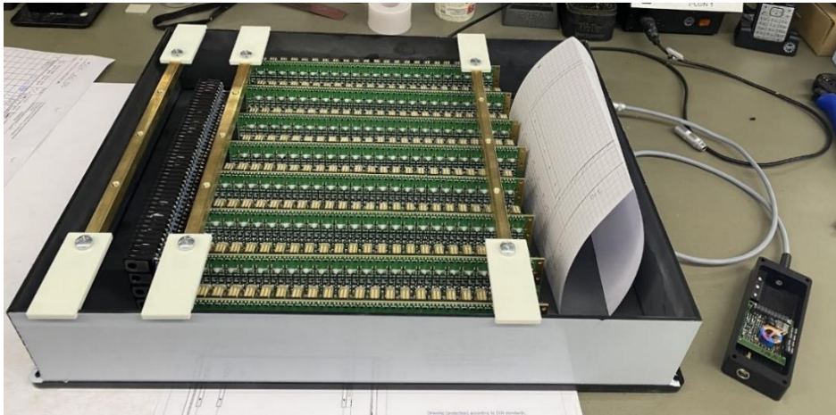
Figure 3.7 – Example of HV Switch during the manufacturing.
