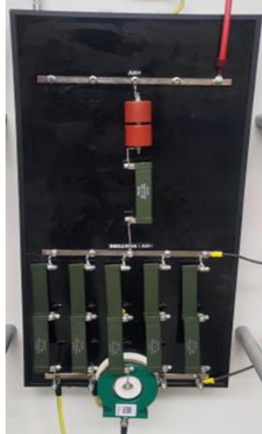
Figure 3.16 – HV SiC Switch with snubber and Distributed load at its terminals.
