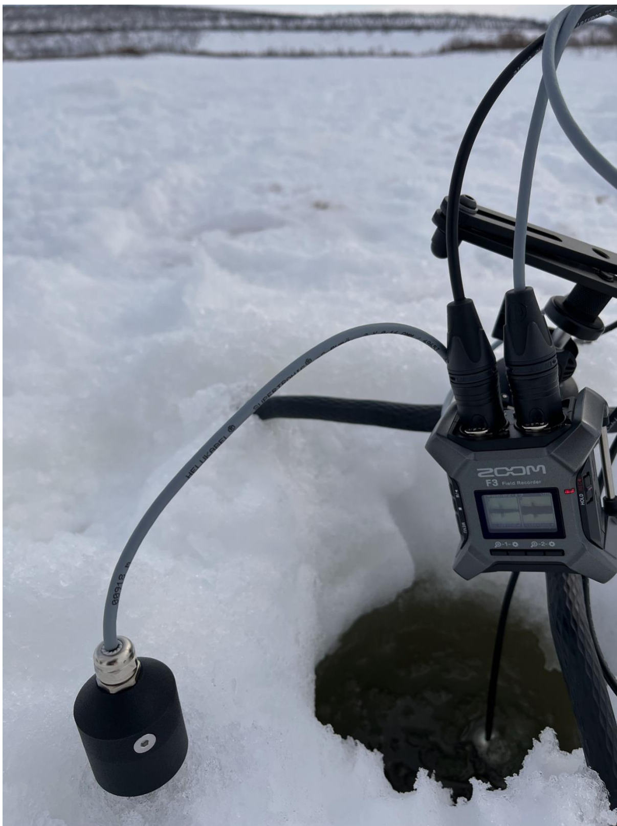
Figure 41 Fishing sounds in Suoidnesuolu, Guovdageaidnu, with a geophonic sensor spiked in the ice and an hydrophone dropped inside an ice-fishing hole.
