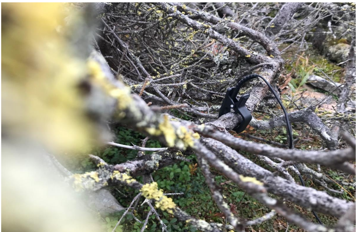
Figure 18 Contact mic clipped to a branch picks up tree-wind interactions on top of Leviduottar, Levi.
