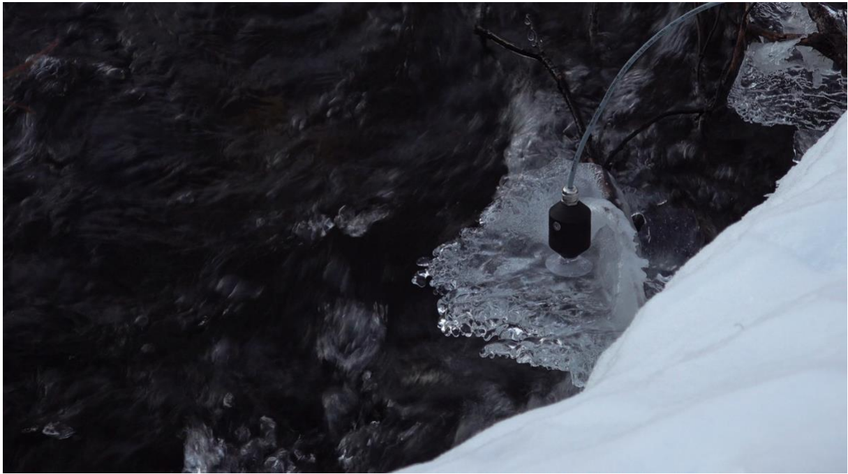
Figure 15 Geophone recording of water running under thin ice at Vuorašjohka, Ávzi.
