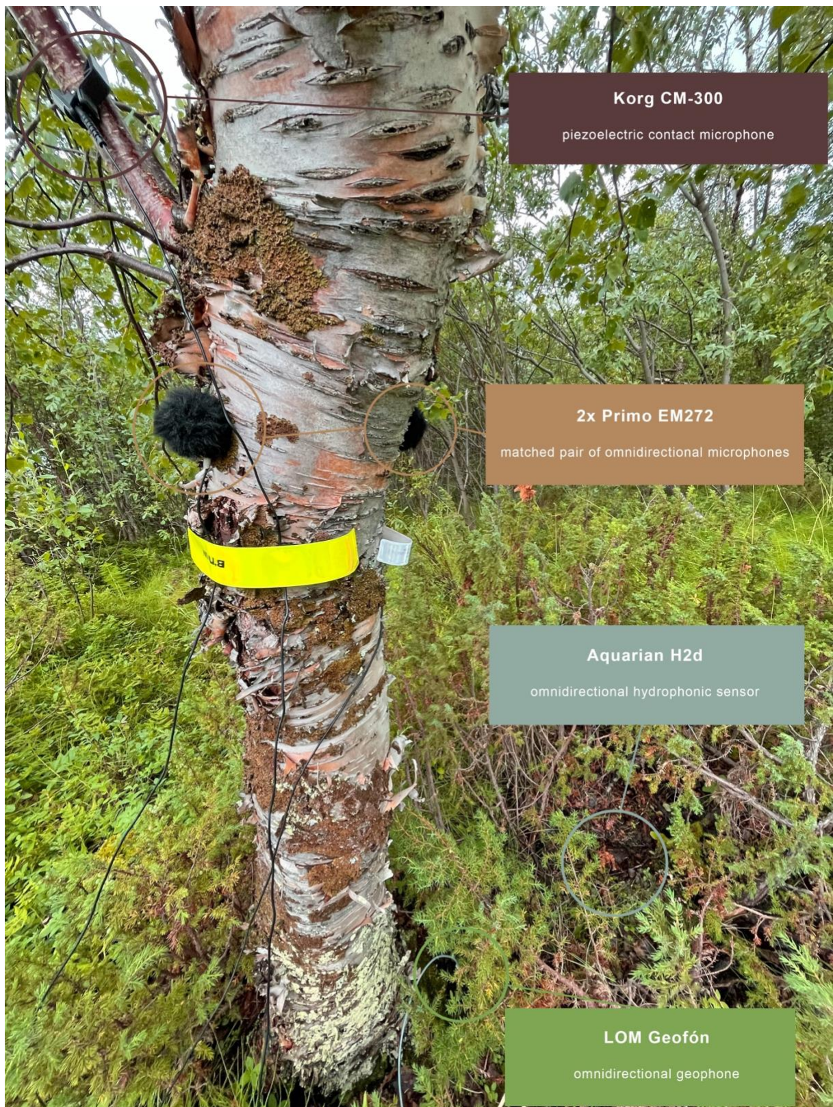
Figure 19 Breakdown of the “Aural Tree” technique, at Buolbmatjávri.
