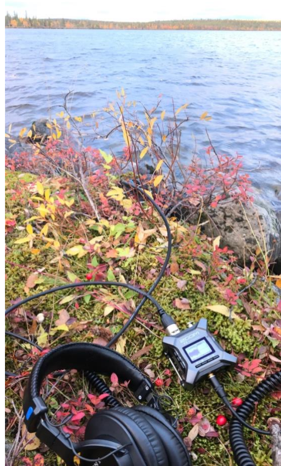
Figure 13 Recording wind-water interactions with hydrophone at Bállásjávri, Muoná.
