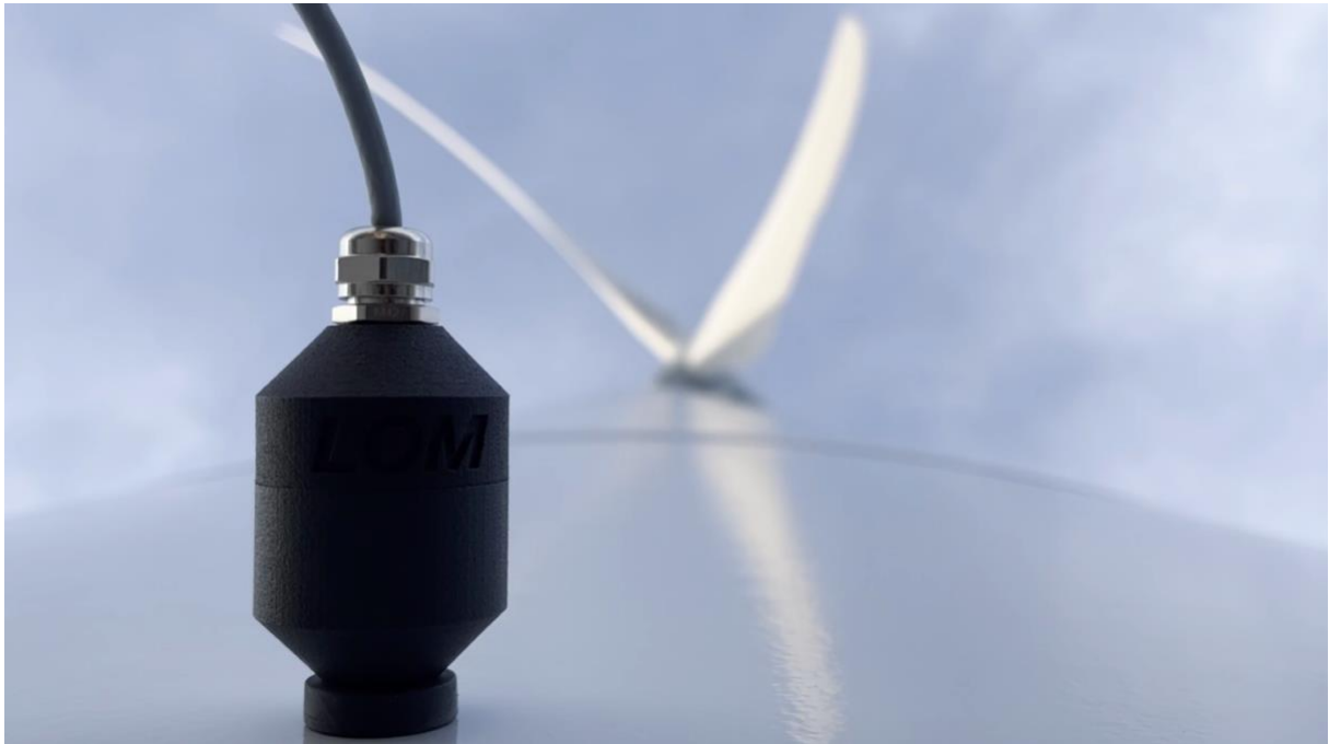
Figure 26 Geophone picking up vibrations from inside the turbine T9, Havøygavlen, Ávvá.
