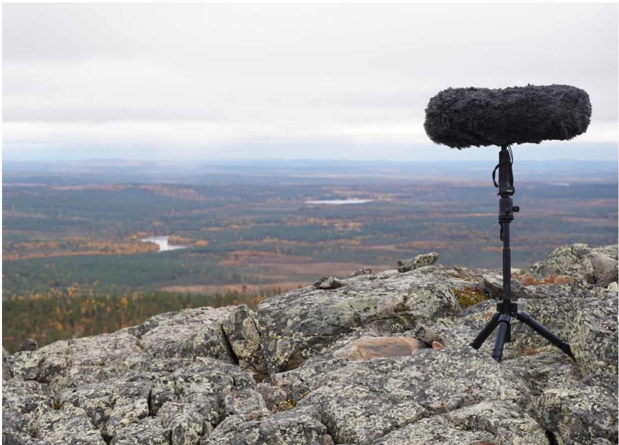
Figure 11 Omnidirectional stereo (A-B) field recording setup at Leviduottar, Levi.
