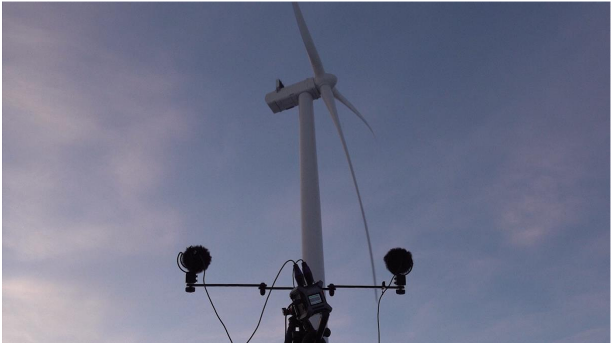
Figure 10 Omnidirectional stereo (A-B) field recording setup at turbine T9, Havøygavlen, Ávvá.
