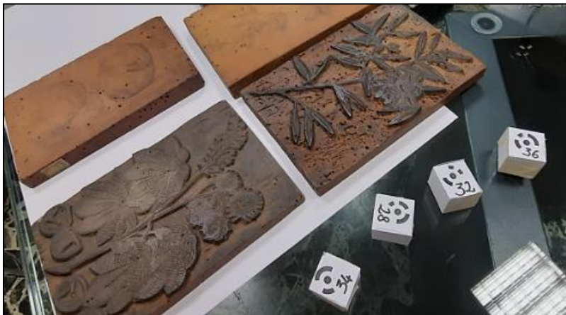
Figure 36. Cube-shaped targets for photogrammetric survey during a survey campaign in Palazzo Poggi collection (Bologna)
