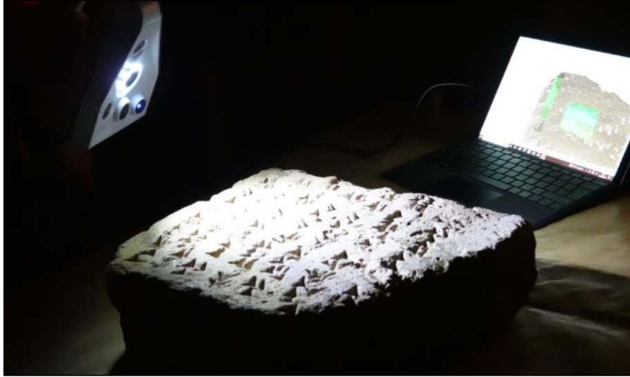
Figure 35. Data acquisition with SLS of an archaeological asset in a dark environment – The artificial external lights were negatively interacting with the projected light pattern.
