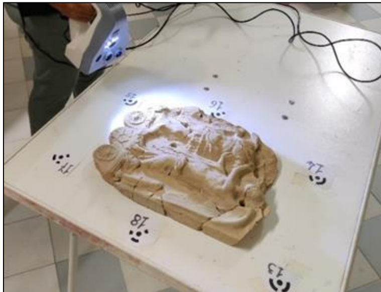
Figure 38. Scanning with SLS in Riccione Museum, capturing the coded targets for registration with DP
