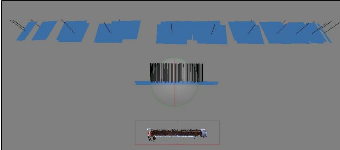
Figure 48. Camera poses as estimated by the SfM software, showing both oblique and nadiral images
