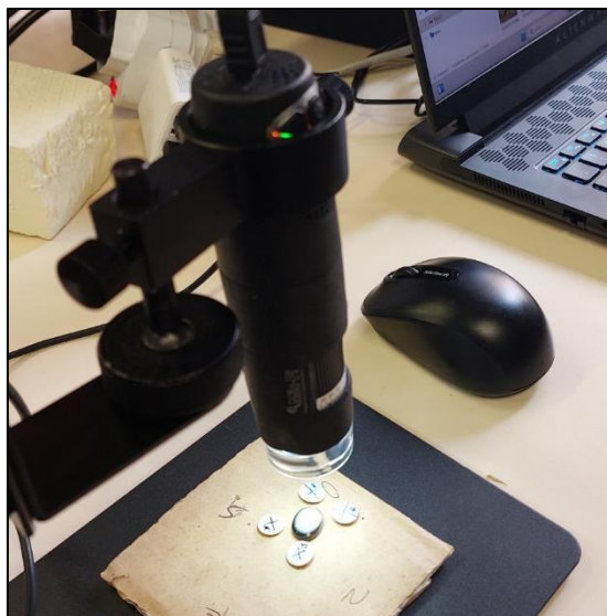
Figure 60. The portable digital microscope acquiring images of the gem
