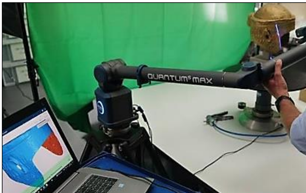
Figure 14. Laser triangulator for museum properties 3D scanning (Patrucco et al., 2023)
