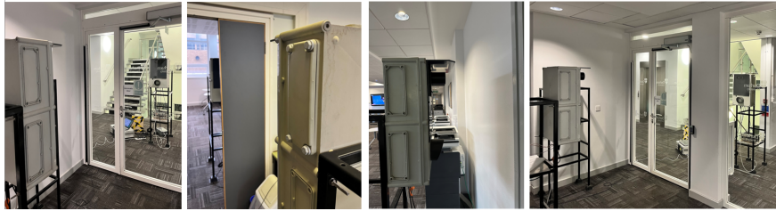
Fig. 5.3 Setup of measurements: Glass door (first), Wooden door (second), Wall partition 1 (third), Wall partition 2 (fourth) [9]
