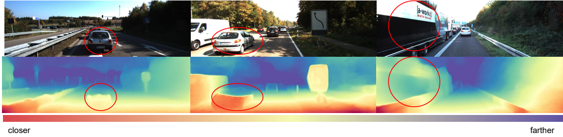
Figure 4.2: Failure cases in self-supervised monocular depth estimation: we employ the existing state-of-art monocular depth estimation network, i.e. LiteMono [220], to predict depth for autonomous driving scenes. It shows unexpected estimation results for moving vehicles.
