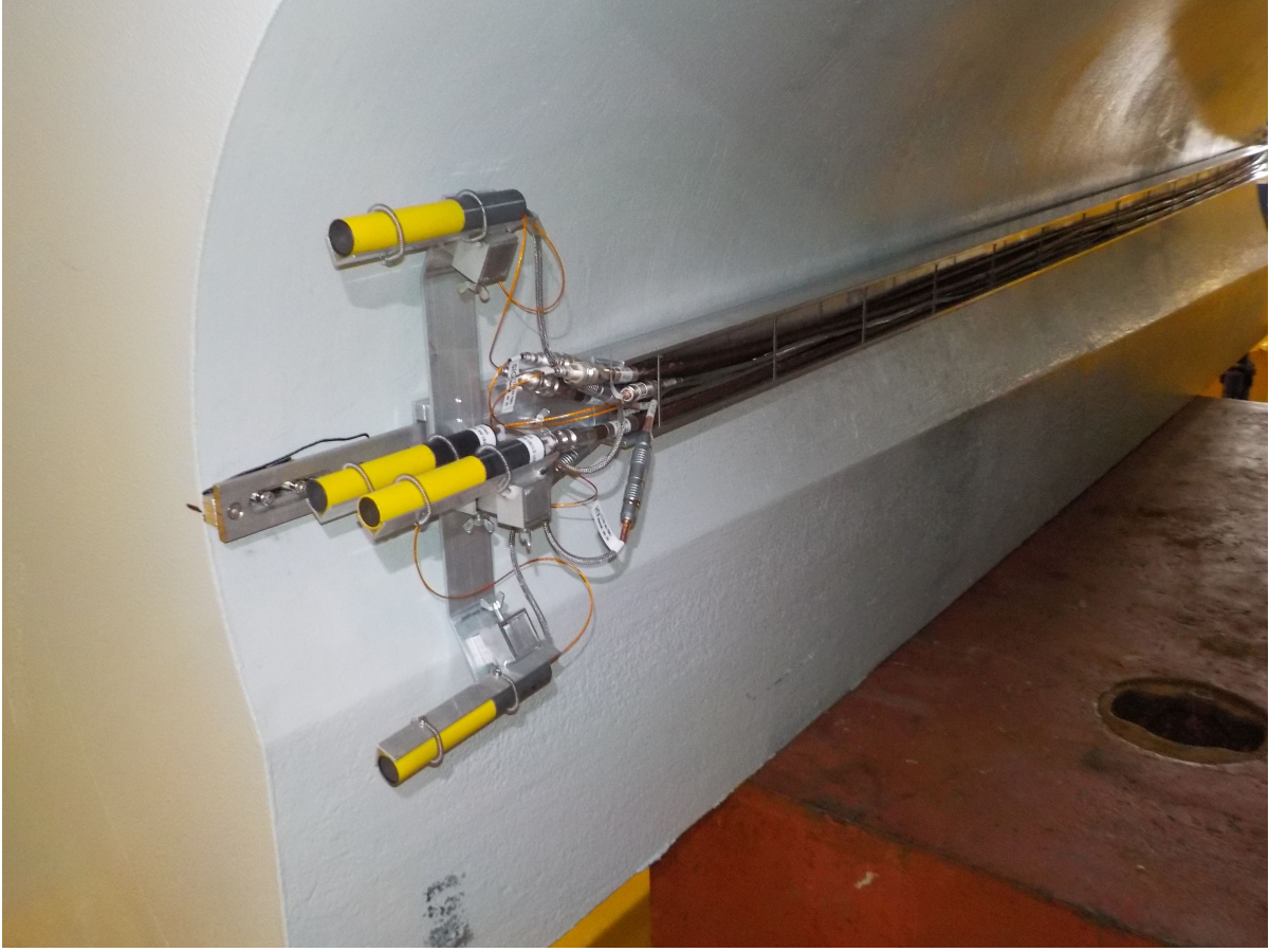
Figure 3.6: Photo of the PMT prototype detector attached to the JFC3 forward shielding.
