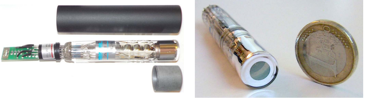
Figure 2.4: Left: Hamamatsu R760 photomultiplier with its base, mu-metal magnetic shield, and a peek cap that seals the ^{207}\text{Bi} source. Right: Modified PMT with a white aluminum ring deposited on the inside of the PMT window.
