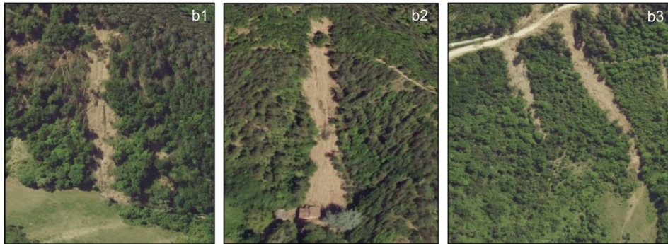
Figure 3.2. Representative images of the two distinct types of debris flows caused by the May 2023 event.
