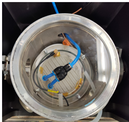
(b) Close-up view of the bio-plasma reactor interior with GAPS inside.
