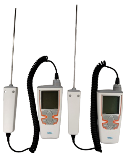
Figure 3.25 – Vaisala HM42PROBE humidity probe used to measure %RH level inside the bio-plasma reactor chamber for FTIR spectra acquisition.
