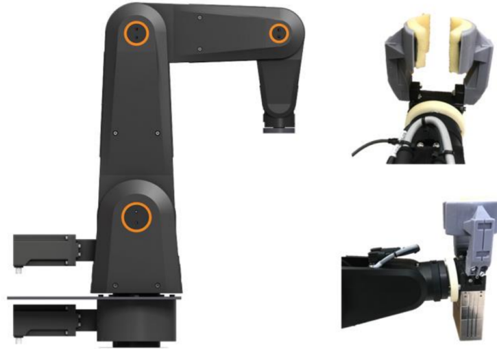
Figure 2.1: Igus RL-DP-5 robotic arm with the customized gripper
