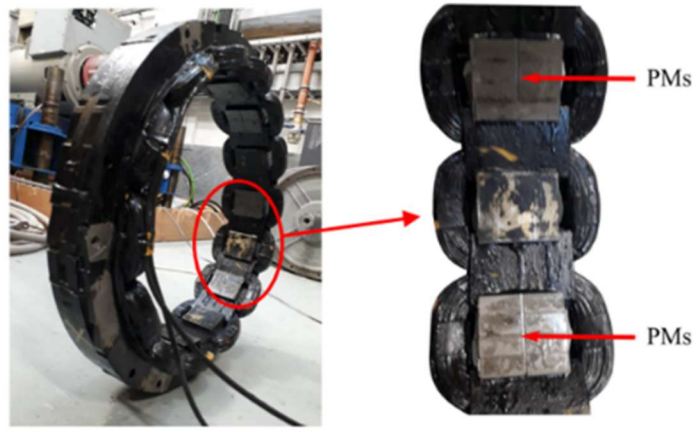
Fig. 95. Hybrid exciter stator highlighting the PM location and layout [85].
