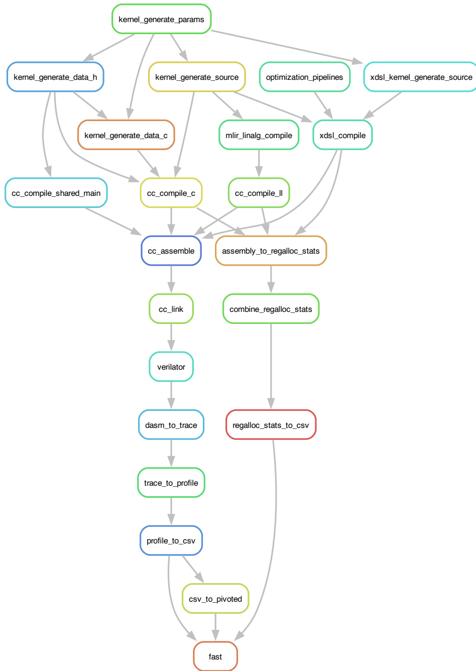
Figure 3.16: Compiler continuous testing and benchmarking pipeline. Vertices represent tasks, edges represent data dependencies. Tasks in the form kernel_generate_* drive the parametric kernel generator to explore the space of input tensor shapes. optimization_pipelines generates variants of the lowering pipeline by incremental addition of optimizations. All tasks downstream of verilator (that runs the actual simulation) are devoted to post-processing of execution traces and computation of performance counters.
