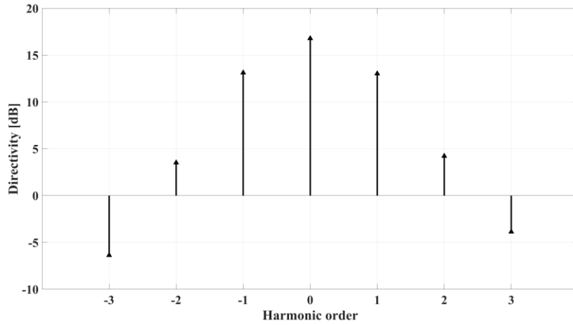
Fig. 39. Maximum directivity at different harmonics.
