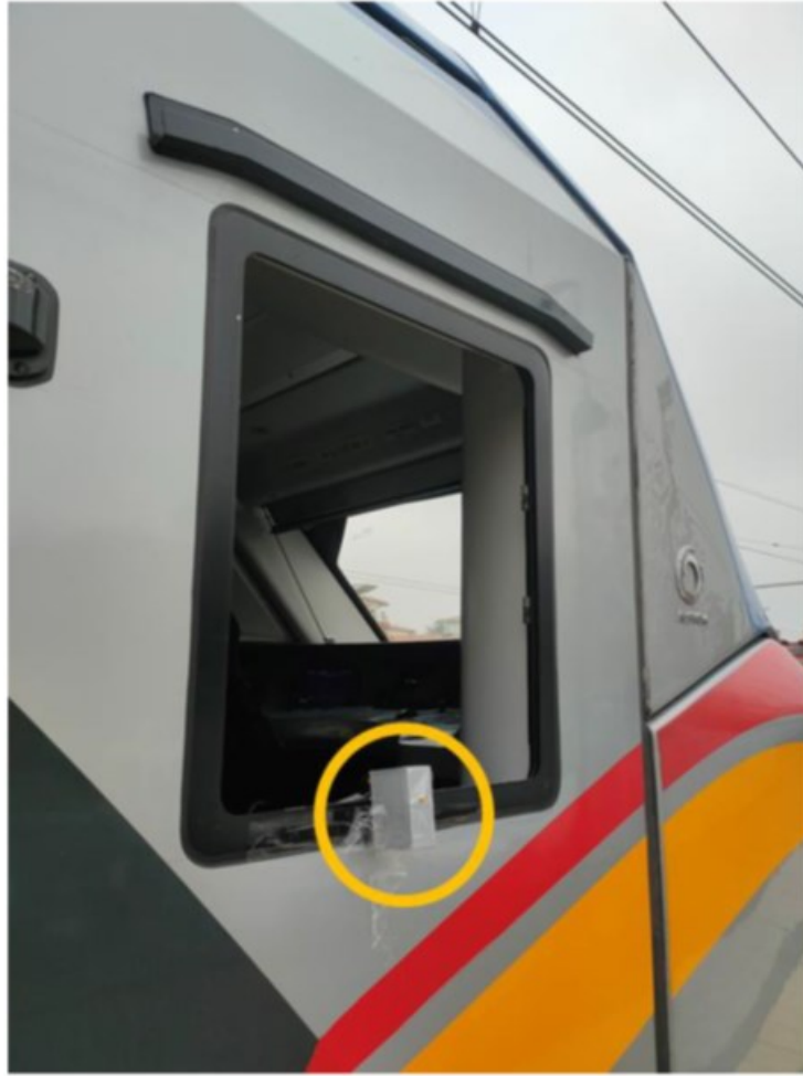
Fig. 56. Positioning of the 2.45 GHz antenna module with PLA case outside the cockpit. © 2024, IEEE
