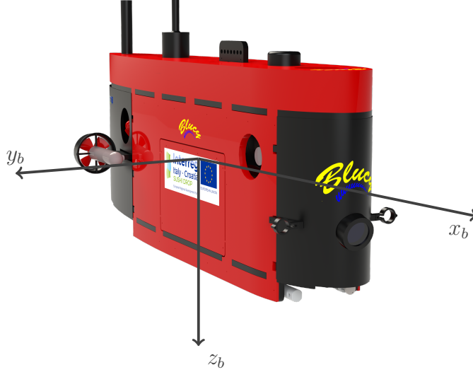
Figure 2.1: The body reference frame of the Blucy.
