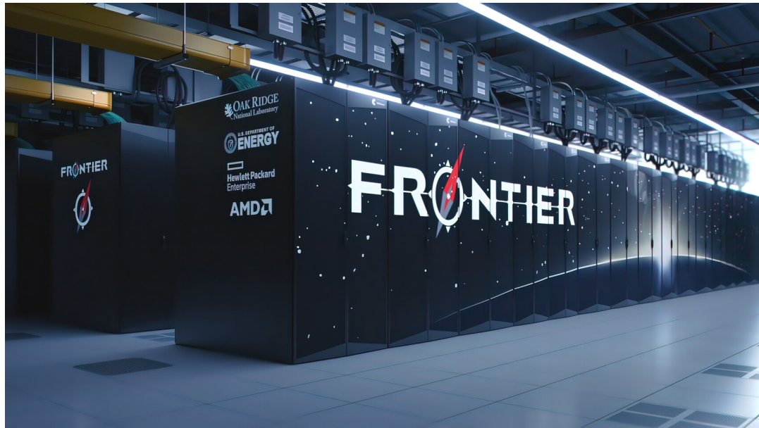
FIGURE 1.3: The Frontier : an exascale supercomputer at the Oak Ridge National Laboratory in the United States, featuring HPE Cray architecture with AMD CPUs and GPUs.
