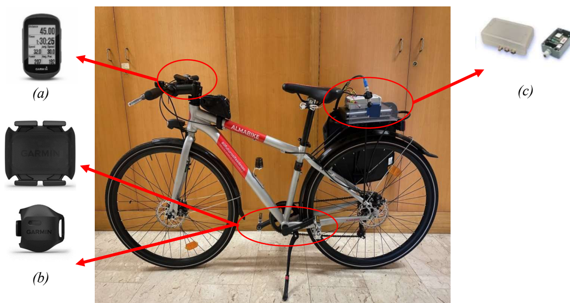
Figure 6-20: Alma Instrumented Bike with all the applied sensors
