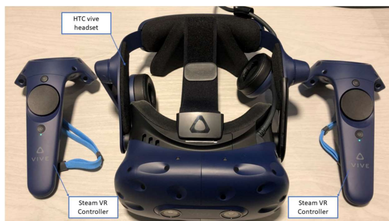
Figure 5-13: HTC Vive Pro Setup and HTC Vive device's components
