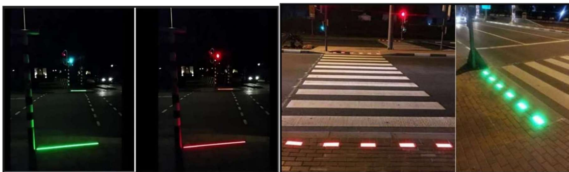
Figure 6-5: a) System with LED strips (left) and b) Smart pedestrian signal (right)
