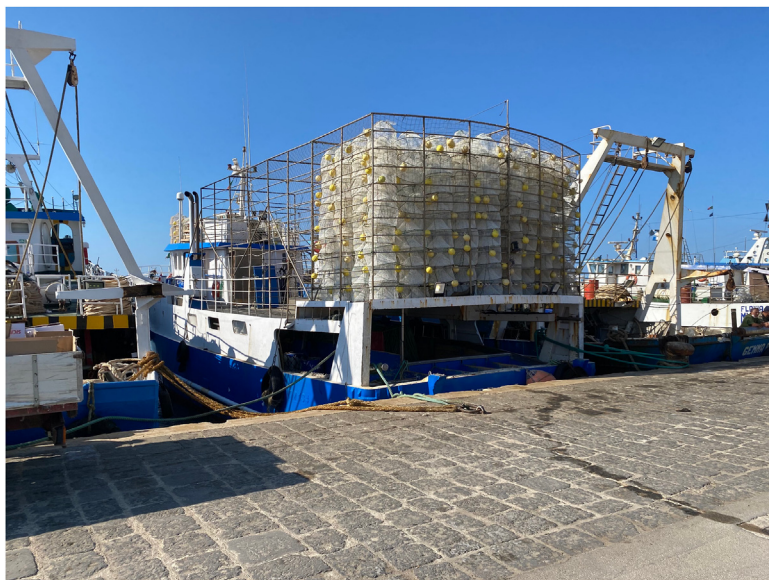
FIGURE 2.5 A Mediterranean fishing vessel (about 30 m of L.O.A.) with a fleet of shrimp traps on the upper deck ready to be set on the main shrimp fishing grounds.
