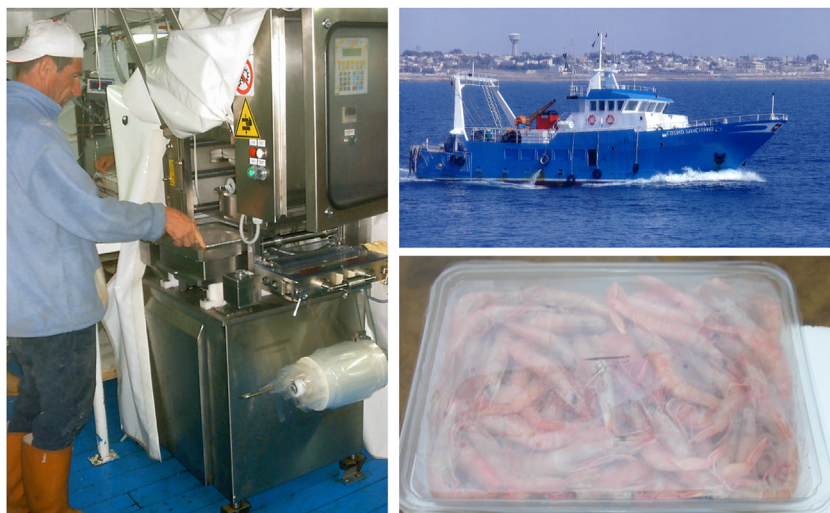
FIGURE 2.10 Onboard packaging of deep-water rose shrimps using a semi-automatic machine for modified atmosphere packaging (100% nitrogen) (Mondini, Brescia, Italy). Shrimps are packed in semi-rigid A.PET/EVOH/PE barrier trays (volume: 1800 cc; laminate density: 1.39 g/cm 3 ; thickness: 500 \mu m) with an oxygen permeability of 1.8 cm 3 /m 2 /day/atm and water vapor permeability of 4 g/m 2 /day (Arcoplastica srl, Andezeno, Italy). The trays are heat-sealed with a multiflex OPP/EVOH/PE film (weight: 72 g/m 2 ; thickness: 75 \mu m) with an O 2 permeability of 3 cm 3 /m 2 /day/atm, a CO 2 permeability of 10 cm 3 /m 2 /day/atm and a water vapor permeability of 3 g/m 2 /day.
