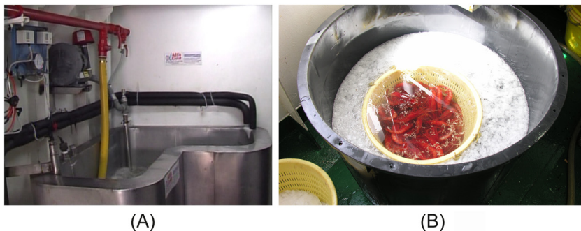
FIGURE 2.12 (A) shrimps hydrocooling machine implemented onboard a Mediterranean bottom trawler; (B) conventional hydrocooling method adopted by small-medium shrimp trawlers. Courtesy of ALFACOLD srl, Italy.
