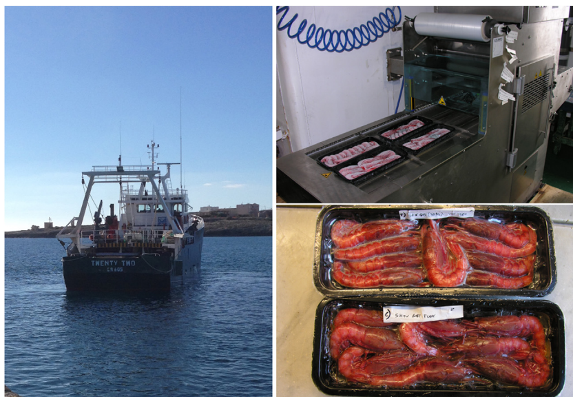
FIGURE 2.11 Automatic onboard packaging of giant red shrimp under skin-vacuum technology. www.facebook.com/gioacchino.bono.980/videos/120396639300418
