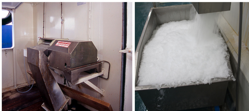
FIGURE 2.14 Flake ice machine implemented onboard a Mediterranean shrimp trawler (LOA: 25–35 m). Courtesy of Frigotecnica soc. coop. (Mazara del Vallo, Italy).
