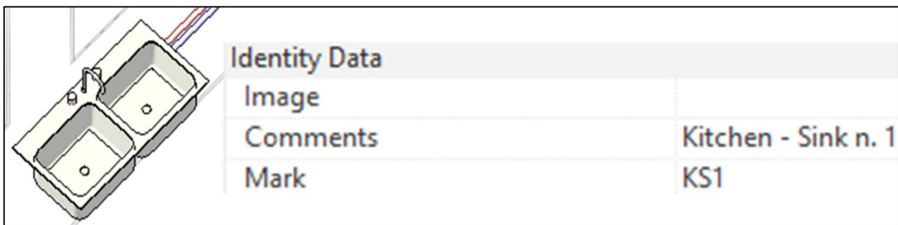
Fig. 20: Sample ID and description related to a sampling point in the properties panel in Revit.
