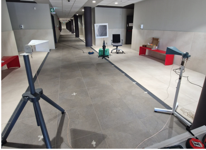
Figure 3.23: Picture of the setup for the RIS 3.47 GHz test. The TX is positioned at a distance of d = 3.75 m, with \theta_i = 3^\circ and \phi_i = 270^\circ . The RX is located 4 meters from the RIS, with \theta_r = 30^\circ and \phi_r = 180^\circ .
