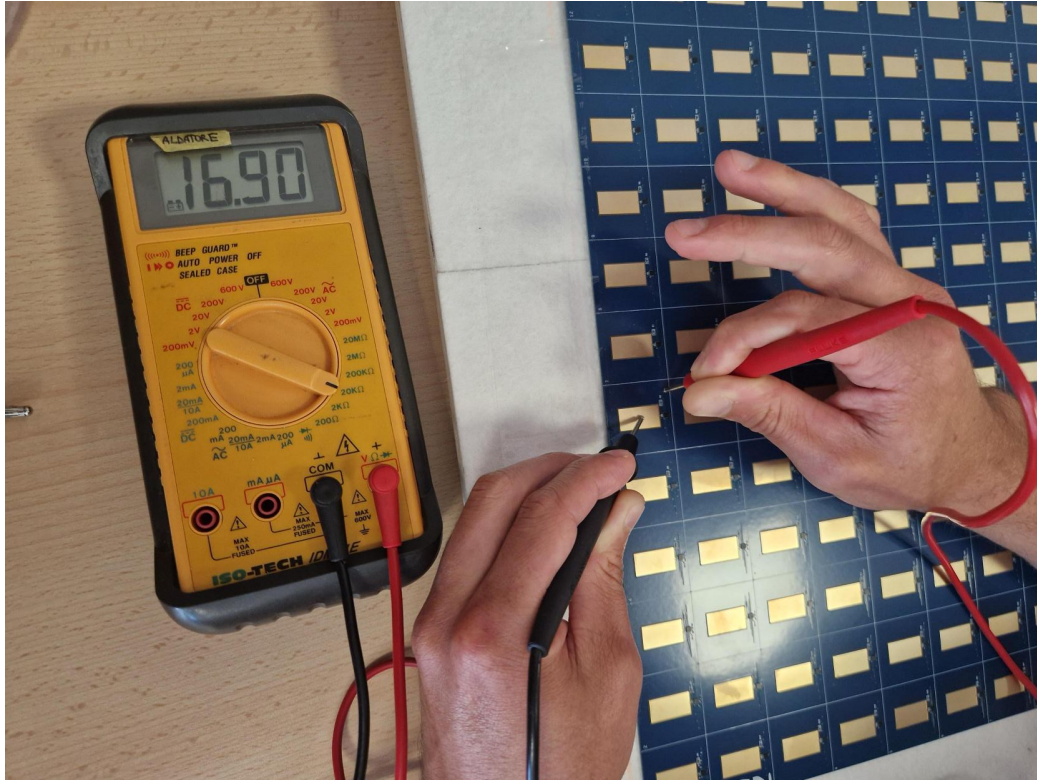
Figure 3.25: Testing each unit cell of the RIS with a voltmeter to ensure that the correct configuration is sent to each cell.
