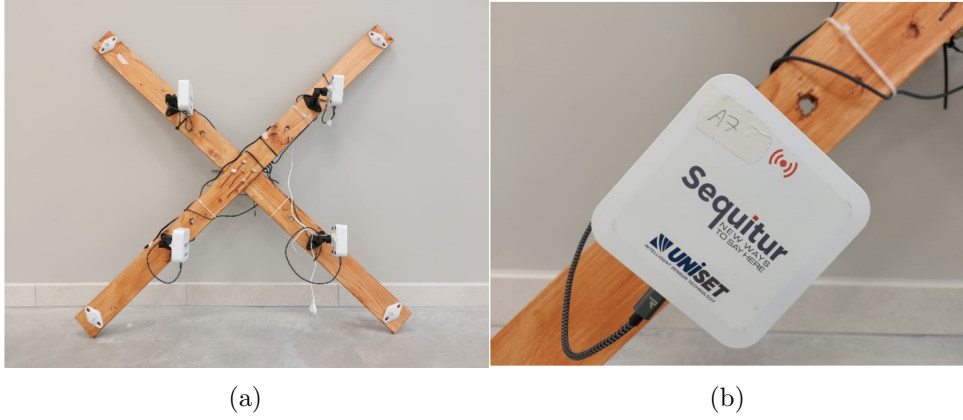
Figure 3.32: Photo of the positioning of the nodes still in a known position (a), close-up photo of the anchor/tag used(b).
