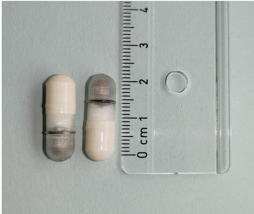
Figure 1. Capsule for Sampling (CapSa) device a rule is included for size comparison.
