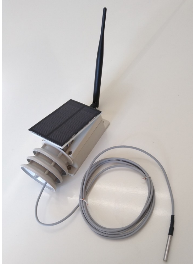
Figure 2.2 Sensor node prototype
