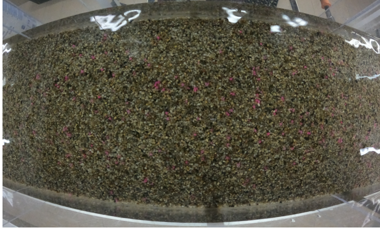
FIGURE 3.4: Example of gravel bed covered by PA6 grains at 1% surface cover. It is visible how the MPs are distributed randomly and uniformly over the bed. The image was not used for further processing.
