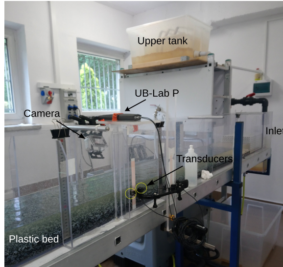
FIGURE 3.2: Experimental setup during PA6 experiments, the transducers for velocity measurements are placed at an intermediate vertical position in the first available cross-section.
