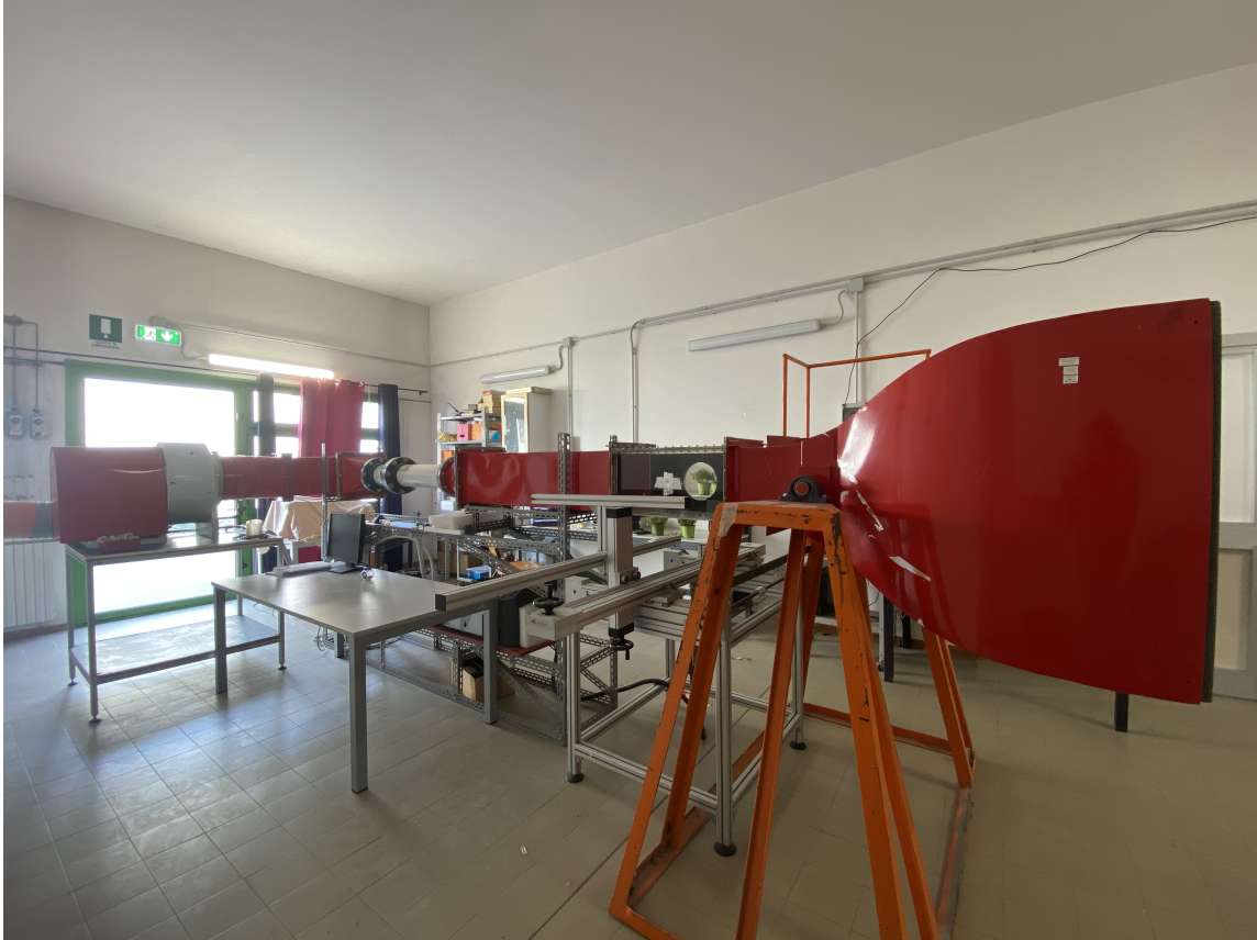
Figure 3.1: wind tunnel used for calculating drag coefficient for crops.
