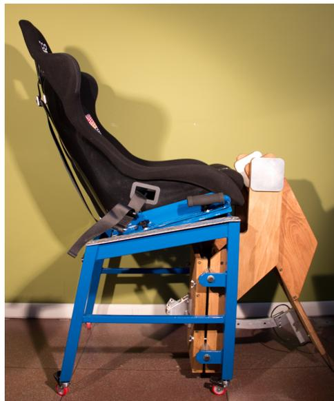
Figure 4.3 Dynamometer chair OT Bioelettronica used for the MVIC test of the healthy adults.
