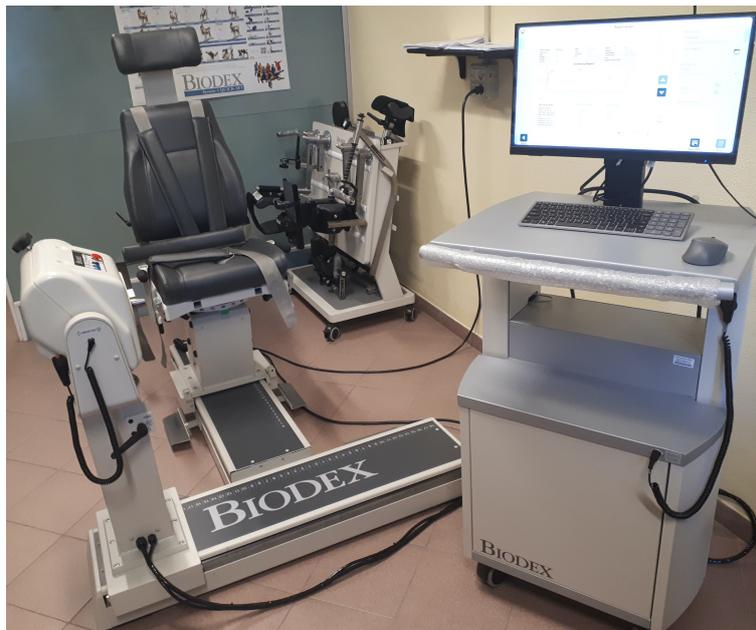
Figure 4.4 Biodex System 4 PRO dynamometer used in the laboratory to acquire torque data with patients.
