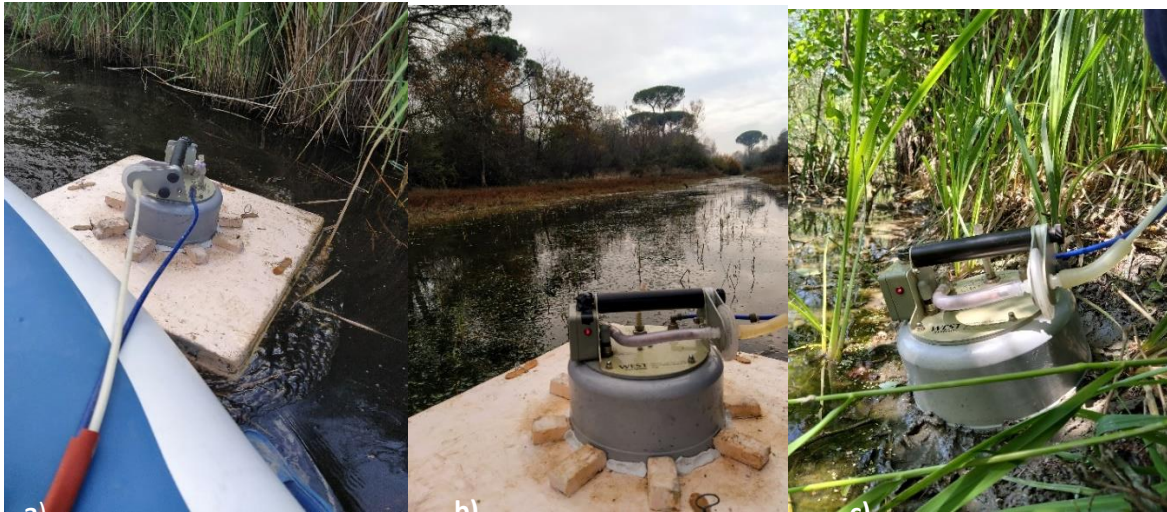
Fig. 2.2 - Measuring GHGs fluxes with accumulation chamber on (a) deep and (b) shallow water with floating device, and on (c) flooded soils.
