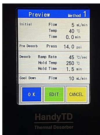
Annex X. 15 Thermal desorption method established for the Handy TD256 after multiple combination tests of the shown parameters.
