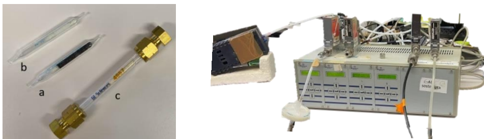
Figure 3. 4 Consumable Anasorb CSC (a) and drying (b) tubes and reusable stainless- steel TA tube (c) (left) and the pumping system (right).
