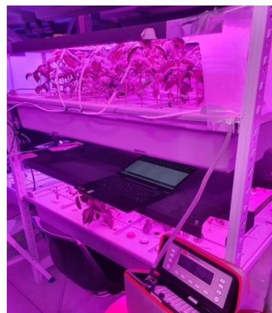
Figure 7. 1 A picture (A.2) of the volatile sampling set-up and its implementation and its simplified representation (A.1): sensors monitoring T&RH (green circle), CO 2 concentration (pink square) and g s (orange star); reintegrated CO 2 (block arrow) and the total air samples taken (line arrows).
