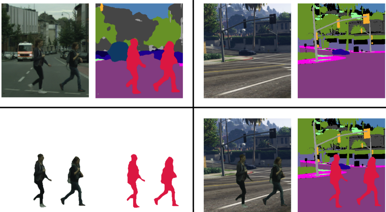
FIGURE 5.3. Given a target image prediction pair (top-left) and a source training pair (top-right), we select classes such as person (bottom-left) and apply our class-wise data augmentation pipeline to synthesise a new training pair (bottom-right). The selected shapes are eroded before being pasted.
