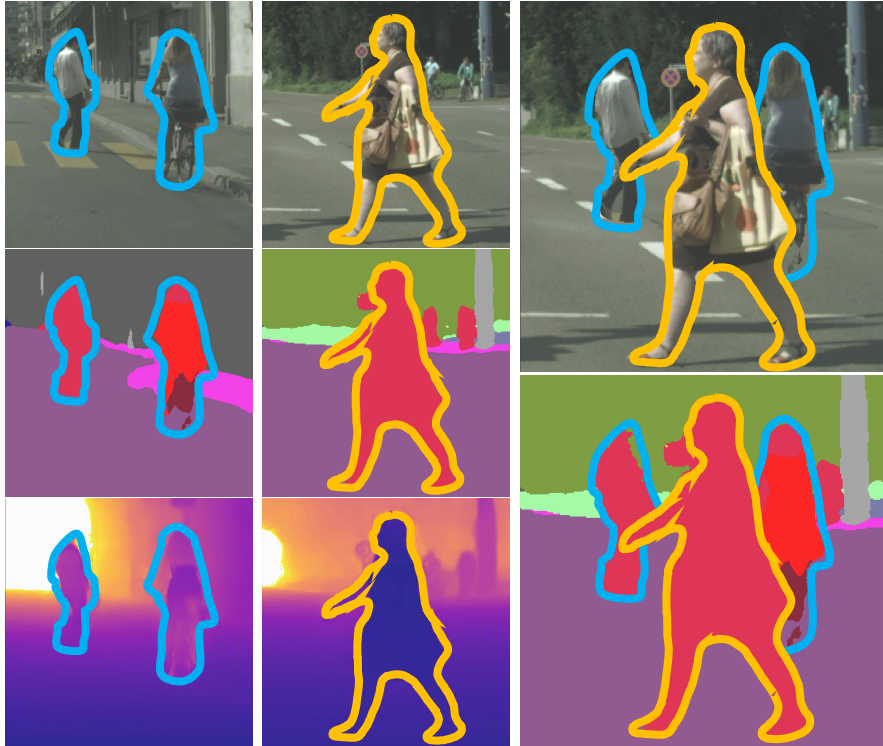
FIGURE 4.4. The rightmost column is a training sample synthesized by copying pixels from left column into the central one. Pixels are chosen according to their semantic class and stacked according to their depths (third row). For example, the two small persons in the left pair are copied behind the one in the middle column. The white pixels in the depth maps represent areas that cannot be copied into other samples due to their depth being too large.
