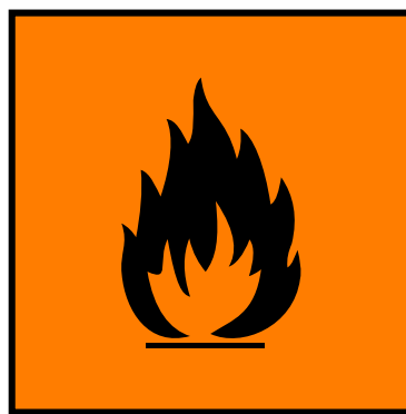
FIGURE 5.4: Example of a highly flammable Hazard symbol.
