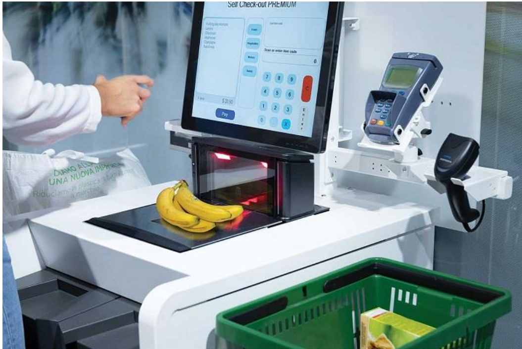
FIGURE 5.6: Examples of a weight-scale used for produce recognition.
