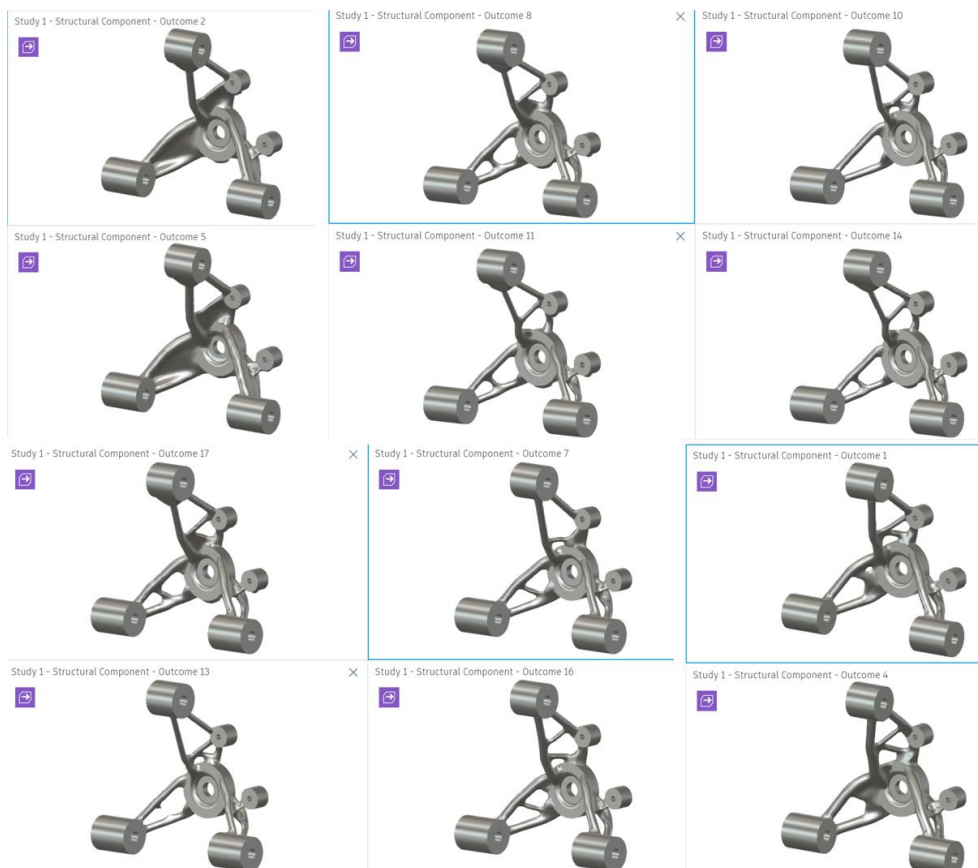
Figure 3.18: Generative design iterative process example
