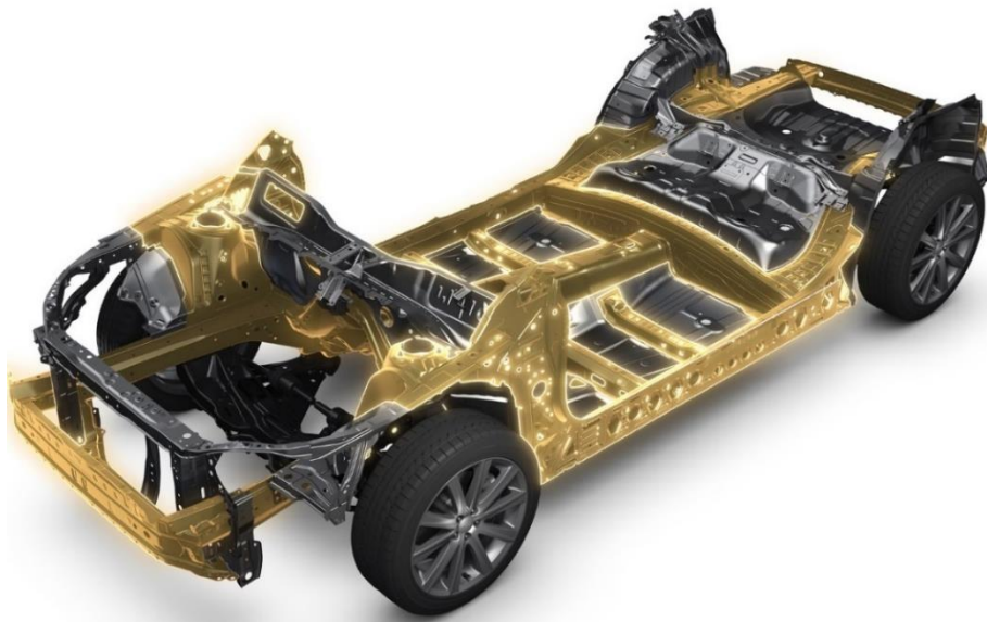
Figure 3.26: Subaru (SGP) modular platform
