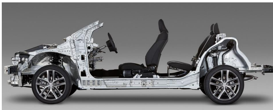
Figure 3.25: Toyota (TNGA) modular platform
