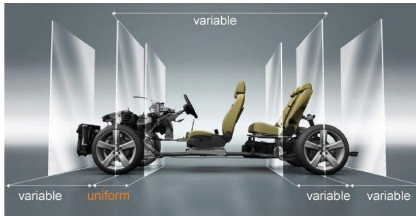
Figure 3.24: Volkswagen MQB modular platform
