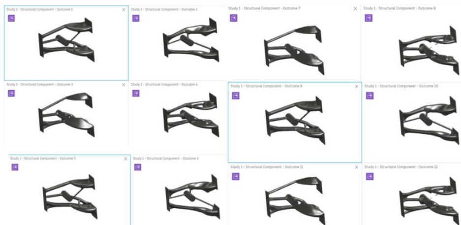
Figure 3.103: Generative design results steel alloys applied Part 4
