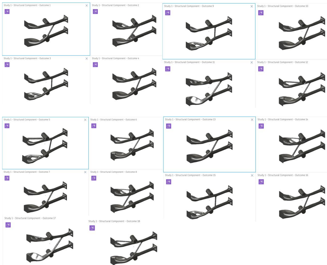
Figure 3.101: Generative design results steel alloys applied Part 1
