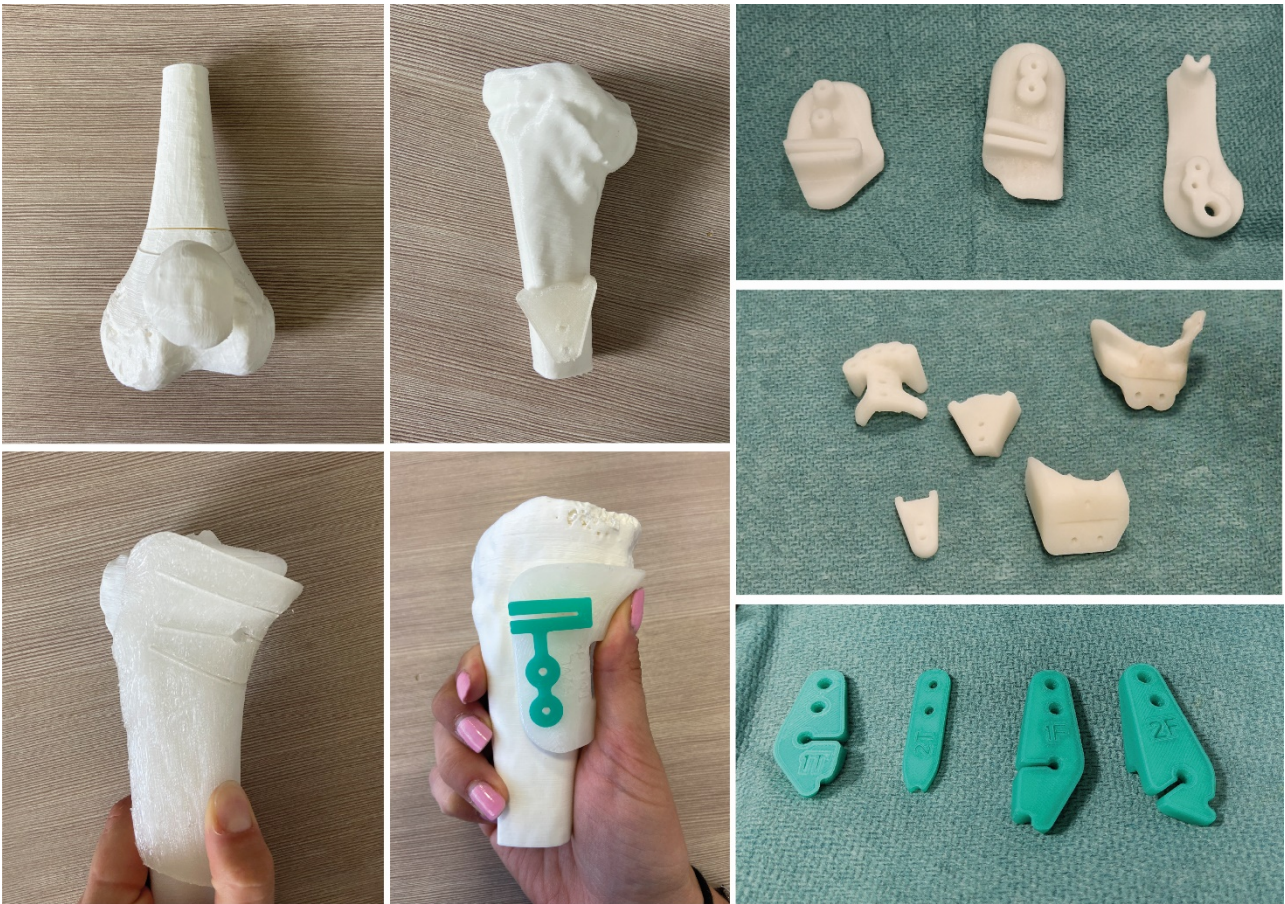
Figure 12. 3D-printed custom-made instruments. These include anatomical models, patient-specific and graft-specific cutting guides, fabricated using opaque PLA, and more translucent Crystal PLA.
