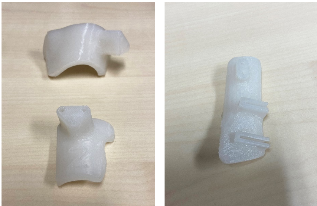
Figure 74. 3D-printed and heat-treated PSIs made of PLA Crystal.
