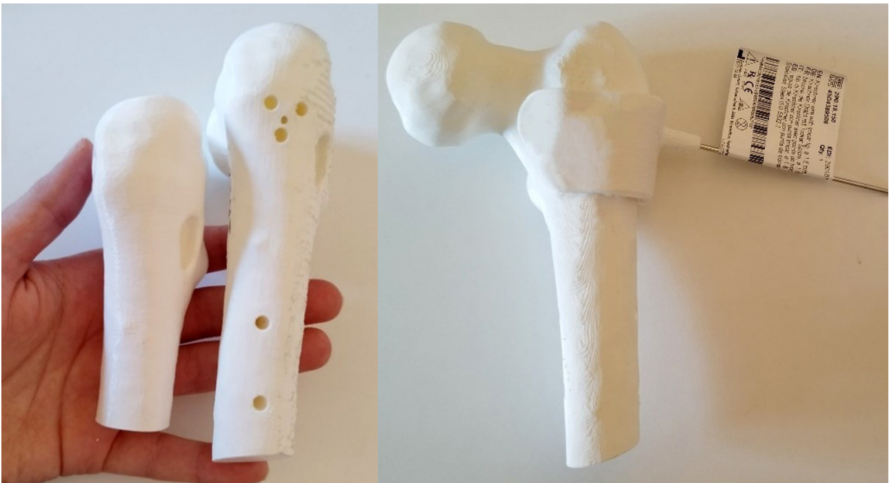
Figure 72. Testing of the proximal PSI on the 3D-printed anatomical model.
