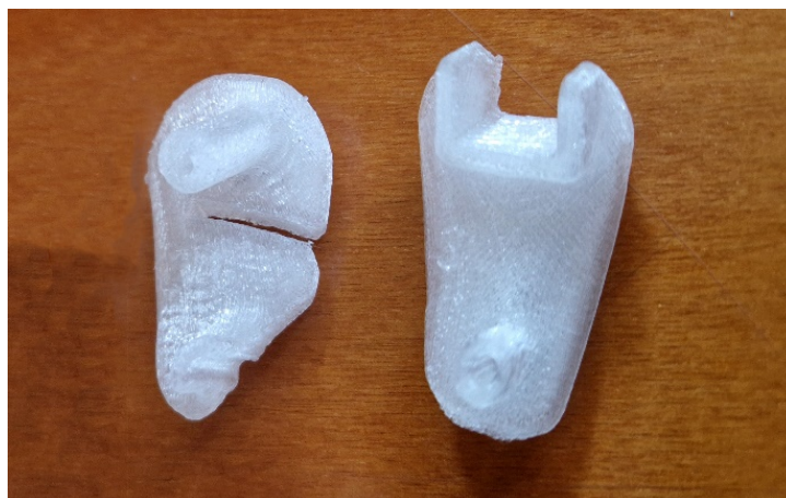
Figure 61. 3D-printed PSIs made of PLA Crystal and heat-treated.
