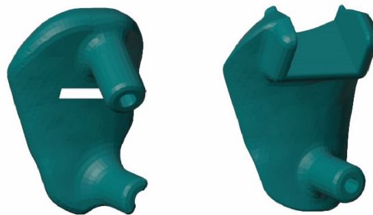
Figure 59. Designed cutting guides. On the left, PSI features two guide wire insertion points - one for plate positioning and one for rotational correction - along with a cutting slot; on the right, the chisel guide is aligned with the plate direction.
