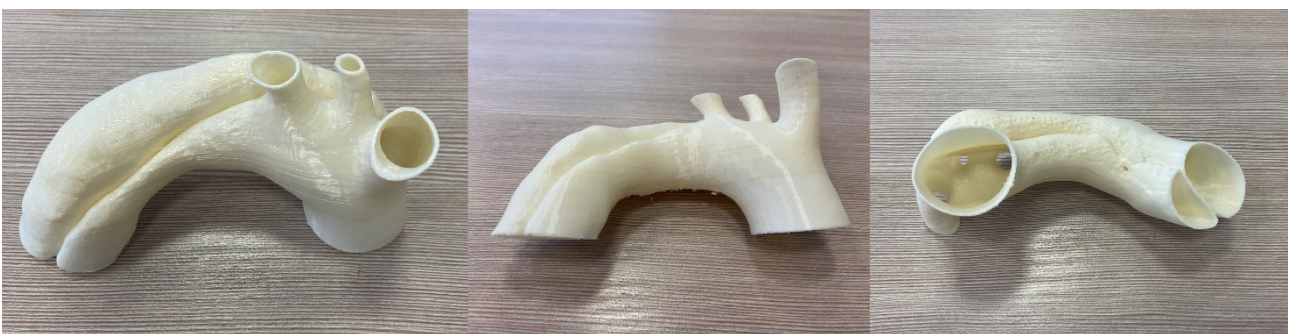
Figure 84. FDM 3D-printed cardiac model in TPU TreeD Pure FT.
