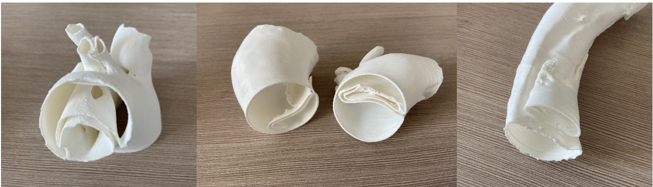
Figure 83. FDM 3D-printed cardiac models in FiloAlfa PLA.
