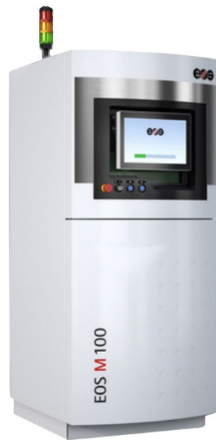
Figure 21. L-PBF 3D printer used: EOS M100.
