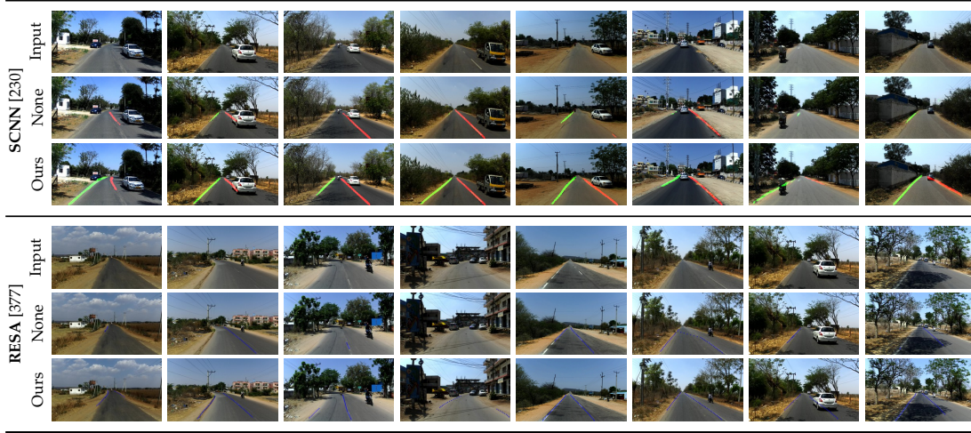
Figure 2.17: Additional qualitative results on lane detection. We train SCNN [230] and RESA [377] on images generated with our method and test on real images with damaged lane markings of IDD [313], improving performances.
