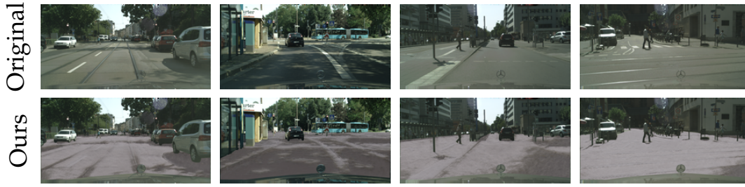
Figure 2.13: Cityscapes images with snow added. We add snow on roads and sidewalks of the Cityscapes training set to train semantic segmentation networks robust to snow. Cityscapes exhibits a domain shift with respect to ACDC, but our method is still able to generate acceptable snow.
