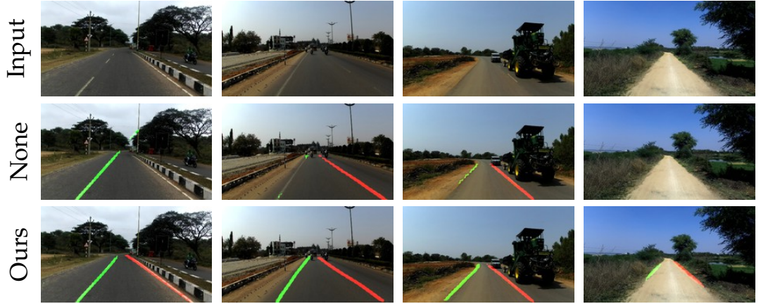
Figure 2.12: SCNN [230] lane detection on IDD [313]. Training on generated images with degraded lanes makes existing lane detectors (e.g. SCNN [230]) resistant to scenes with damaged (first three columns) or no (last column) lane markings.
