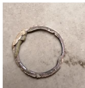
Figure 18 Picture reporting the appearance of membranes and o-rings before and after permeation.
