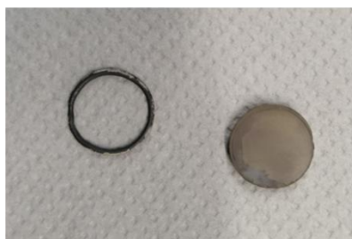
Figure 18 Picture reporting the appearance of membranes and o-rings before and after permeation.
