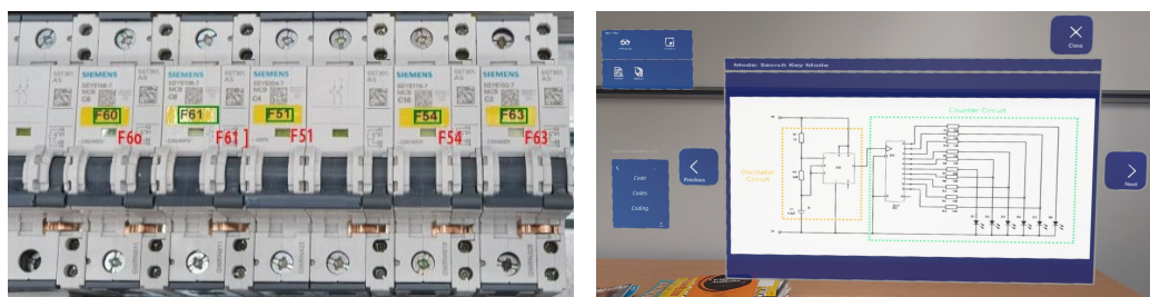
(a) Deep learning-based OCR applied to physical electrical board codes. (b) AnnHoloTator: Key-Search Mode linked to the OCR retrieved code.
