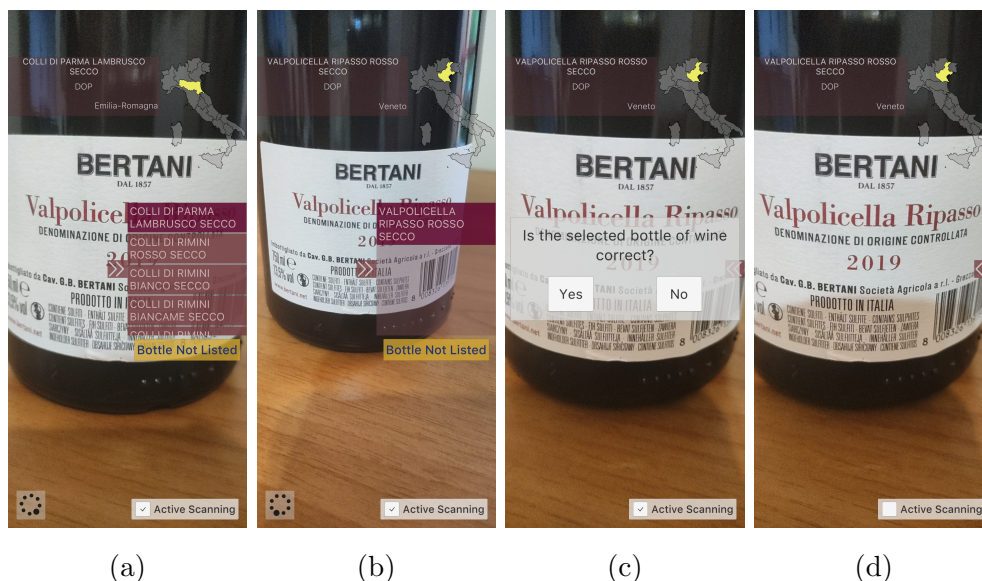
Figure 4.22: AR interface: (a)-(b) Wrong and Correct results, (c) Correct confirmation, (d) After the confirmed identification, the scan stops.
