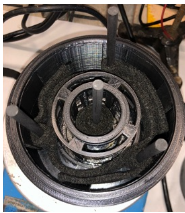
Fig.15 Picture of the 3D-printed fuel cell with cylindrical design. The picture includes the fuel cell body, the removable supports, and the electrodes: 3 rods encircled by a felt ring at the anode and 1 rod encircled by a felt stripe at the cathode.
