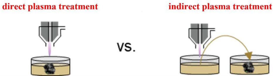
Figure 1.2-2 Schematic representation of direct and indirect plasma treatment. Figure adapted from
