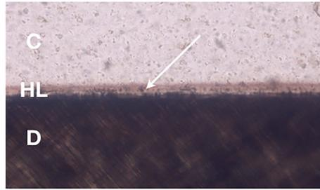
**Figure 29.** Representative light microscopy images (20x magnification) of the tested materials in the experimental conditions and submitted to nanoleakage with silver nitrate after 24 h of storage in artificial saliva (T0). D = Dentin; HL = Hybrid Layer; C = Composite. Arrows indicate areas of silver nitrate particles deposition.
