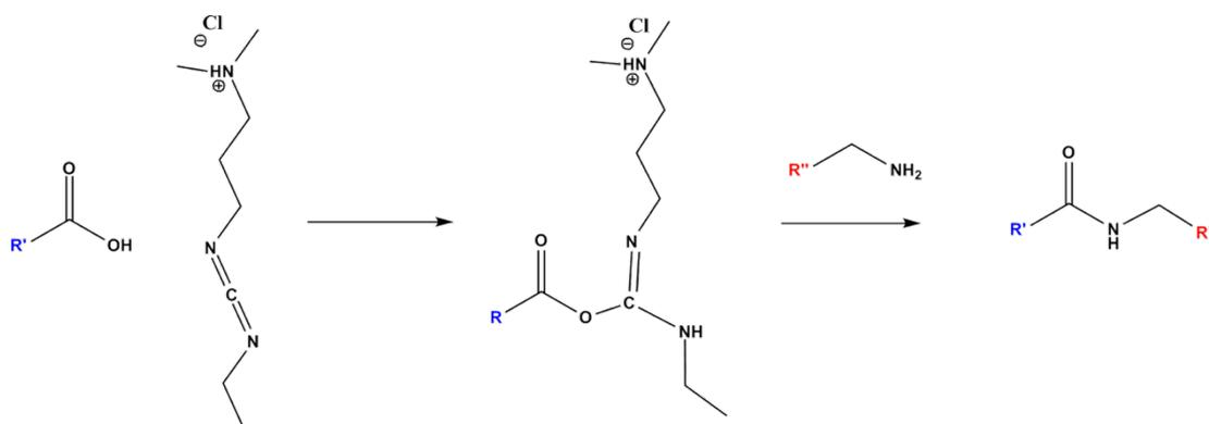
**Figure 8.** EDC cross-linking reaction: EDC reacts with carboxylic group of, after the elimination of O-acylisourea intermediate, the glutamic or aspartic acid bond the N residue of lysine or hydroxylysine.
