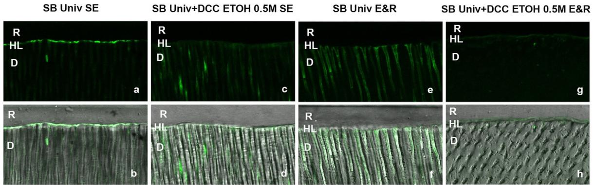
**Figure 17:** Representative examples of in-situ zymography of the resin-dentin interfaces at T0. Dentin treated with SBU adhesive in the SE mode (a, b); SBU (SE) + DCC 0.5M (c, d); SBU in the ER mode (e, f); SBU (ER) + DCC 0.5 M (g, h). D: dentin; HL: hybrid Layer; R: resin composite.
