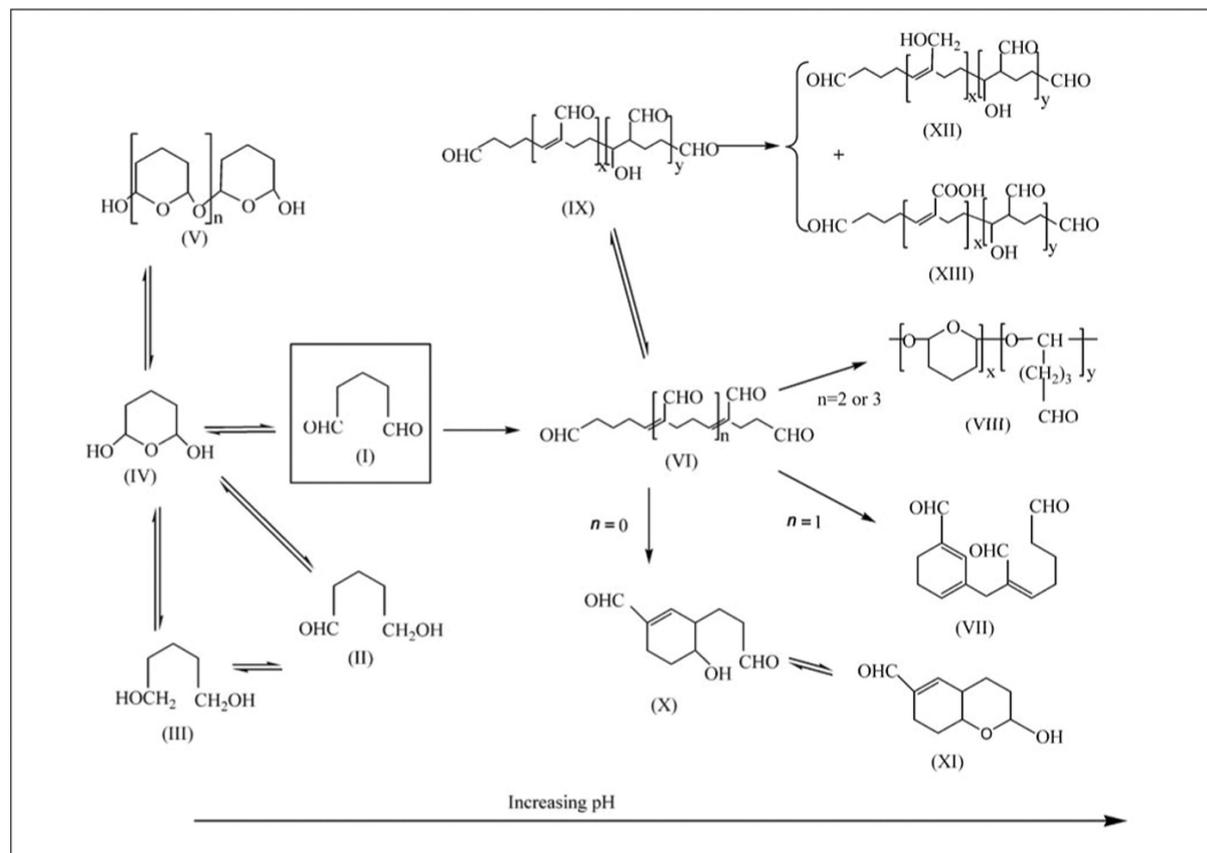
**Figure 6.** Summary of the possible forms of glutaraldehyde in aqueous solution.
