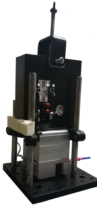
Figure 5.3: Photo of the laboratory setup used for the NIR spectra acquisition.
