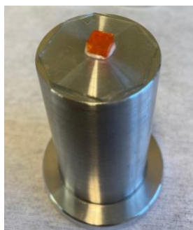
Figure 2.6 Picture of a \text{MAPbBr}_3 single crystal glued to the support for polishing, at CEA, Grenoble. Courtesy of Javier Mayén Guillén.
