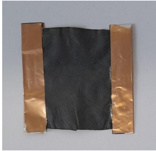
Figure 64: Optical image of rGO-coated PA6 electrospun mat with silver paint/copper foil electrical contacts
