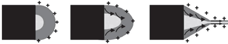
Figure 3: Schematic of core-sheath nanofiber formation [7]
