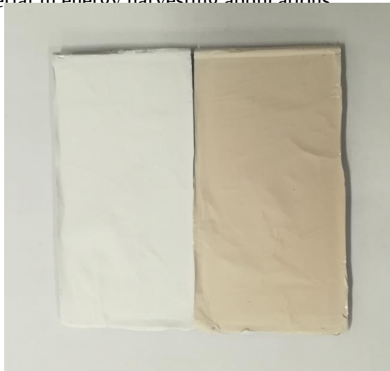
Figure 38: Optical images of PVdF and PVdF/GO 0.5% electrospun mats
