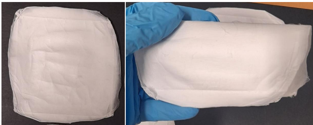
Figure 51: Optical image of electrospun PA6 mats highlighting its flexibility
