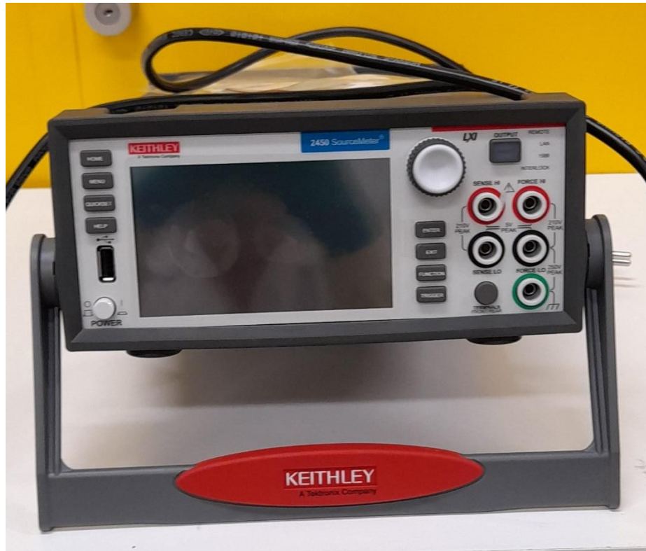
Figure 28: The Keithley multimeter used for the acquisition of electrical conductivity measurements
