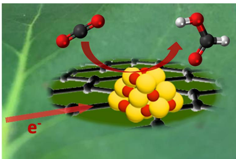
Figure 1.5 Graphic illustration of the CO 2 reduction to formic acid on CeO 2 nanoparticle supported by MWCNTs.
