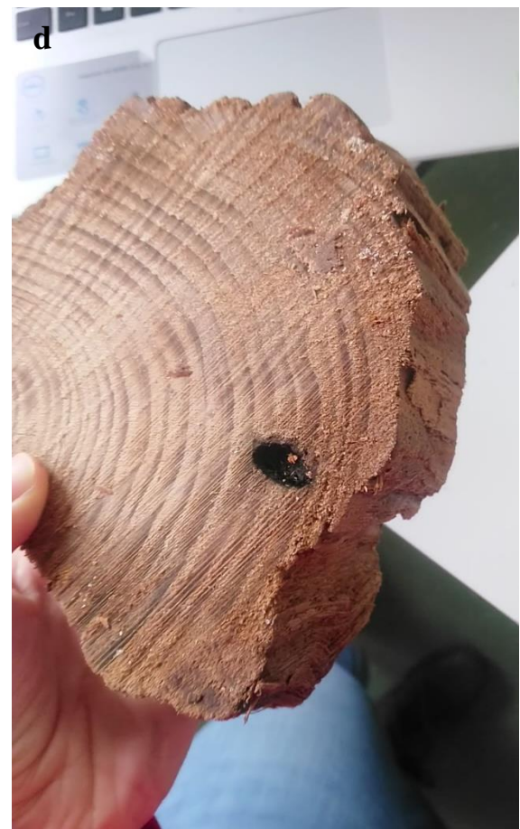
Fig. 29 Discolorations and charcoals on the cross-section and on the outermost area
