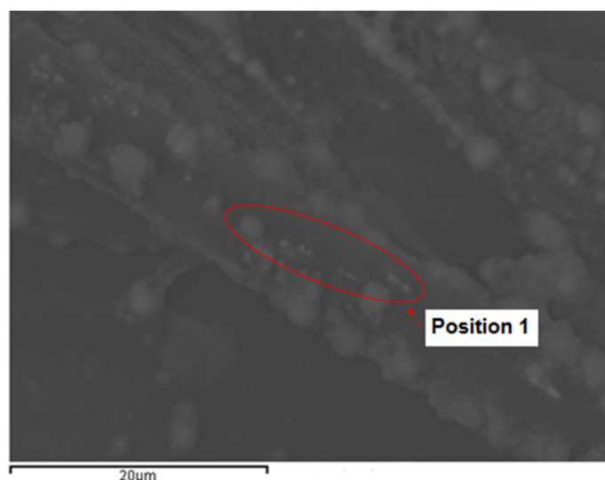
Figure 3.14. SEM images of the CuMgAl LDH/CP reduced in 0.1 M KNO 2 at 333K for 1h and 30 min
